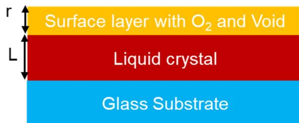
Figure 8. The optical model used to extract the optical constants of liquid crystalline thin films.
