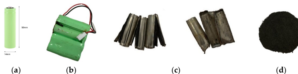
Figure 7. Spent NiMH batteries (a) The size of the typical NiMH battery, (b) Cases of spent cells, (c) Housings and small plastic parts, (d) Black battery mass.
