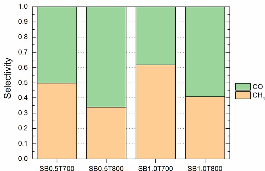
**Figure 5.** Selectivity for commercial Ni/Al<sub>2</sub>O<sub>3</sub> catalyst considering all the gasification conditions (S.B0.5T700 means a syngas produced using an S/B ratio of 0.5 and a gasification temperature of 700 °C).
