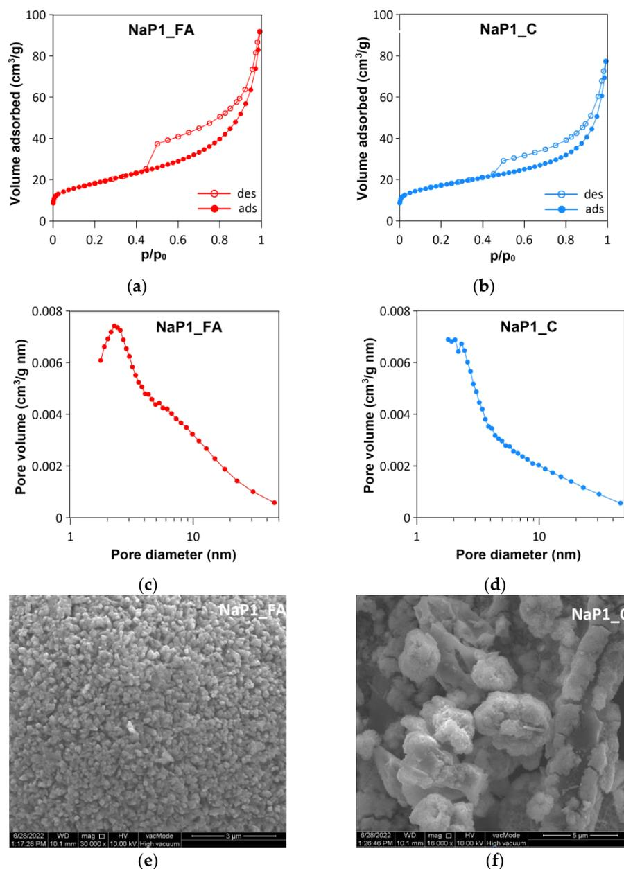
**Figure 3.** Textural analysis of NaP1\_FA and NaP1\_C samples: (a,b) N<sub>2</sub> adsorption/desorption isotherms, (c,d) pore size distribution diagrams, and (e,f) SEM microphotographs.
