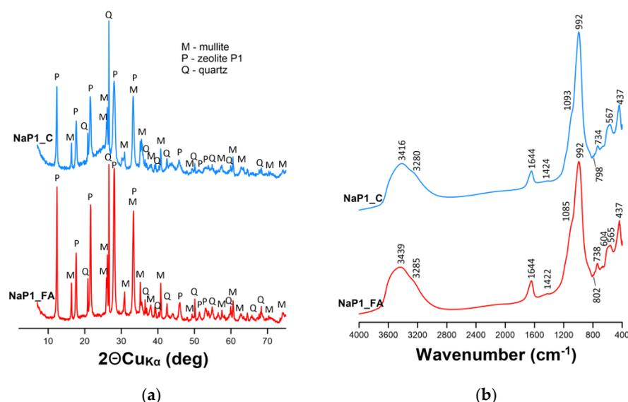
**Figure 1.** (a) X-ray diffraction patterns and (b) Fourier transform infrared spectra of NaP1\_FA and NaP1\_C samples.
