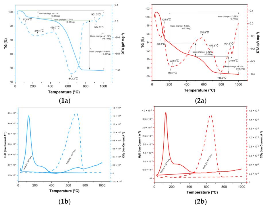
Figure 2. Thermal curves of (1) NaP1\_C and (2) NaP1\_FA [(a) TG/DTA, (b) QMS].
