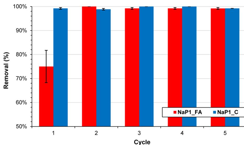
**Figure 9.** The EA removal efficiency of NaP1\_FA and NaP1\_C after regeneration cycles.
