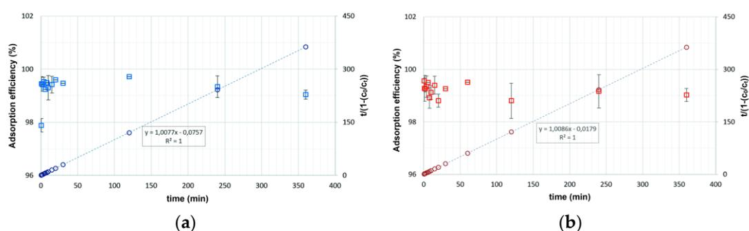
**Figure 8.** BMG kinetic models for the adsorption of EA on (a) NaP1\_C and (b) NaP1\_FA.
