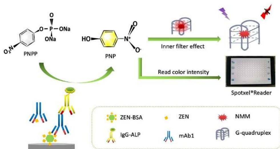
Figure 2. Schematic illustration of the fluorescence and colorimetric dual-mode immunoassay for detection of ZEN based on G4/NMM [64]. Copyright 2023 Elsevier.
