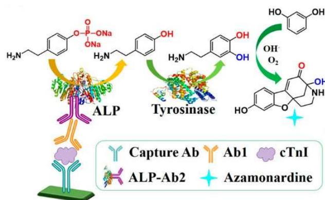
Figure 5. Schematic representation of the cascade ELISA strategy via tandem enzymatic fluorogenic and chromogenic reactions [75]. Copyright 2018 American Chemical Society.
