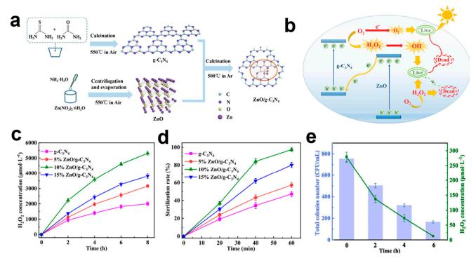
**Figure 6.** (a) Synthetic process of the  $ZnO/g-C_3N_4$  heterojunction photocatalyst. (b) Pathway of  $H_2O_2$  production and photocatalytic sterilization. (c)  $H_2O_2$  productivity under simulated sunlight over various catalysts. (d) Sterilization efficiency for bacteria over different photocatalysts. (e) Residual sterilization performance after the photocatalytic process [110]. Copyright 2021, Elsevier.
