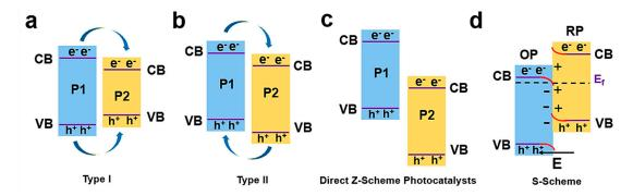
**Scheme 4.** Schematic representation of the traditional (a) Type-I, (b) Type-II, (c) Z-scheme, and (d) S-scheme electron transfer paths.
