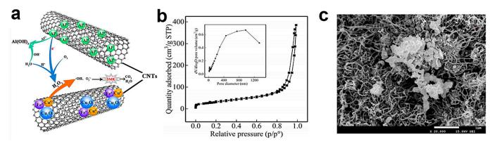
**Figure 2.** (a) The reaction mechanism of the  $Al^0$ -CNTs-Fe-Cu/O<sub>2</sub> system. (b) N<sub>2</sub> adsorption/desorption isotherm and the pore size distribution (the inset) of CNTs-Fe-Cu. (c) SEM image of the CNTs-Fe-Cu composite [108]. Copyright 2020, Elsevier.
