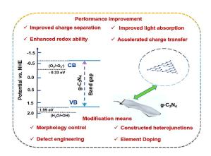
**Scheme 3.** Schematic representation of the modification of the photocatalytic self-Fenton system based on the g- $C_3N_4$  photocatalyst.
