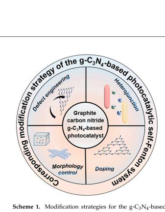
**Scheme 1.** Modification strategies for the g- $C_3N_4$ -based photocatalytic self-Fenton system are briefly described.
