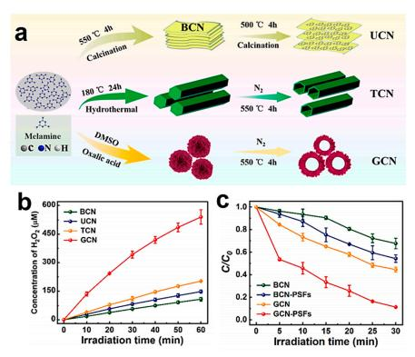
**Figure 3.** (a) Synthesis schematic diagram of g- $C_3N_4$  with four different morphologies (BCN, UCN, TCN, and GCN). (b) Photocatalytic  $H_2O_2$  production of BCN, UCN, TCN, and GCN under visible light irradiation. (c) The photocatalytic decomposition curves of 2,4-DCP with BCN, BCN-PSFs, GCN, and GCN-PSFs under visible light irradiation. Reproduced with permission [114]. Copyright 2022, Elsevier.
