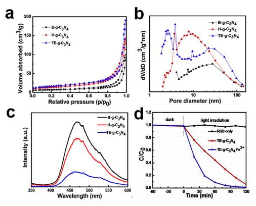
**Figure 1.** (a) Nitrogen adsorption–desorption isotherms and (b) Barrett–Joyner–Halenda (BJH) pore size distribution plots for the B-g- $C_3N_4$ , H-g- $C_3N_4$ , and TE-g- $C_3N_4$  samples, respectively. (c) Photoluminescence PL spectra of B-g- $C_3N_4$ , H-g- $C_3N_4$ , and TE-g- $C_3N_4$ . (d) Removal efficiency of RhB using TE-g- $C_3N_4$  [107]. Copyright 2020, Elsevier.
