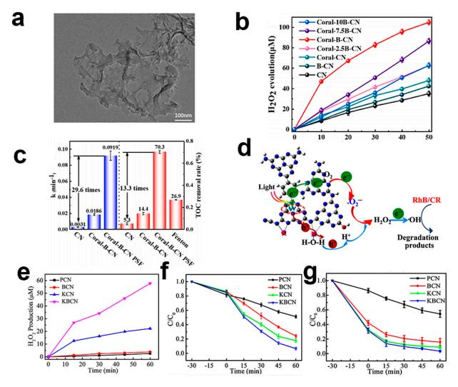
**Figure 8.** (a) TEM image of coral-B-CN. (b)  $H_2O_2$  yield curves for different catalysts. (c) The k-value and TOC removal rate for different systems [122]. Copyright 2023, Elsevier. (d) Schematic of Fenton-like degradation of RhB and CR with in situ-generated  $H_2O_2$  over KBCN. (e) Photocatalytic production of  $H_2O_2$  in pure water. Results of the degradation efficiencies (f) for RhB and CR (g) over KBCN [117]. Copyright 2022, Elsevier.
