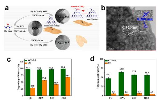
**Figure 4.** (a) Schematic diagram of the formation process of the as-prepared catalysts. (b) HR-TEM images of KCN-0.5. (c,d) Degrading efficiencies and the TOC removal rates of organic pollutants by KCN-0.5 and CN. Reproduced with permission [125]. Copyright 2023, Elsevier.
