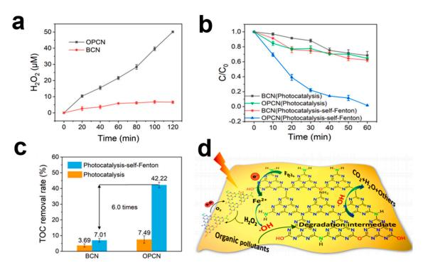
**Figure 9.** (a) The photocatalytic  $H_2O_2$  generation curves of BCN and OPCN. (b) The 2,4-DCP degradation activity. (c) The TOC removal rate between photocatalysis-self-Fenton and photocatalysis based on OPCN and BCN. (d) Schematic illustration of the photocatalysis-self-Fenton system based on OPCN [24]. Copyright 2022, Elsevier.
