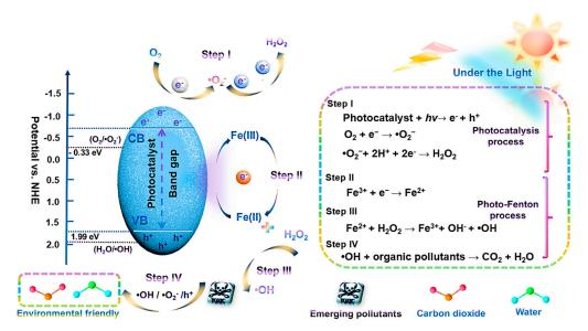
**Scheme 2.** Schematic diagram of the mechanism of the photocatalytic self-Fenton system for the degradation of emerging pollutants.
