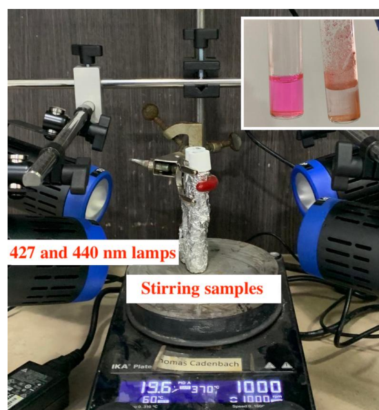
Figure 9. Setup of a photocatalysis experiment.
