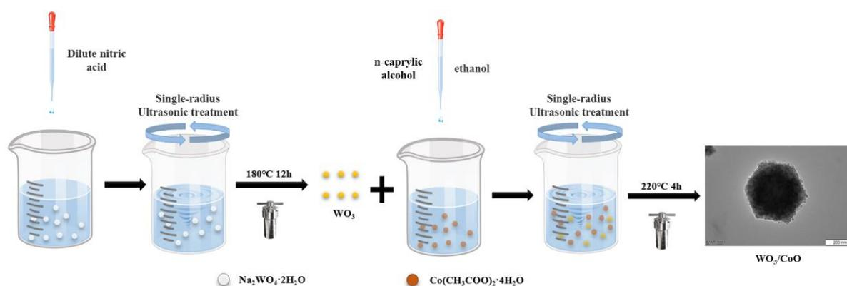
**Figure 10.** Schematic diagram of synthesis for as-prepared photocatalysts.
