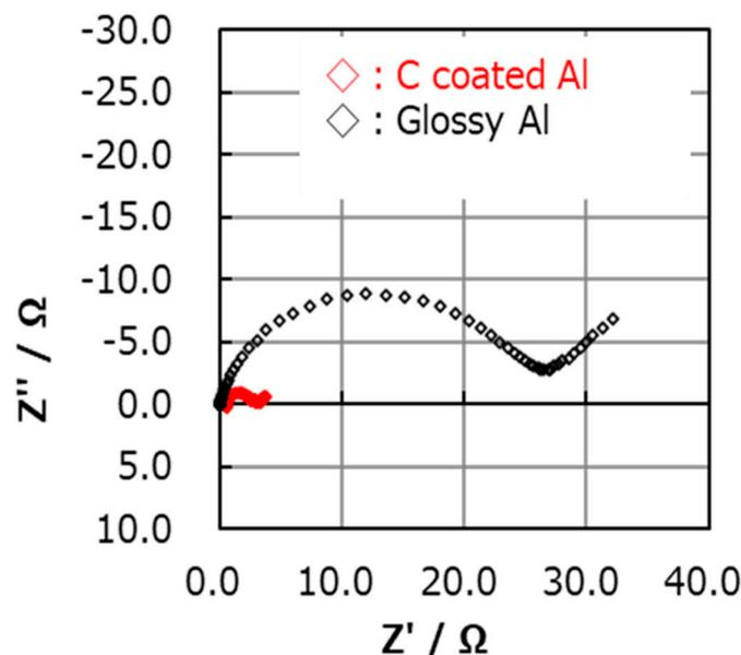
**Figure 2.** Initial impedance spectra of composite sulfur electrodes (presented as Nyquist plots from 0.1 Hz to 1 MHz) with glossy and carbon-coated current collectors. 7/2/1 S/super P/ PEO component with 1.3 mg/cm<sup>2</sup> sulfur loading and 1 M LiTFSI in 1:1 DOL/DME.
