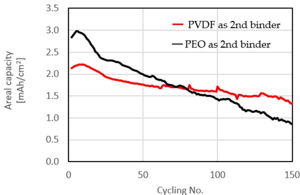
**Figure 6.** Cycling performance of cells comprising cathodes with high sulfur loading with different binders for the interface between the two components of the composite cathode [4].
