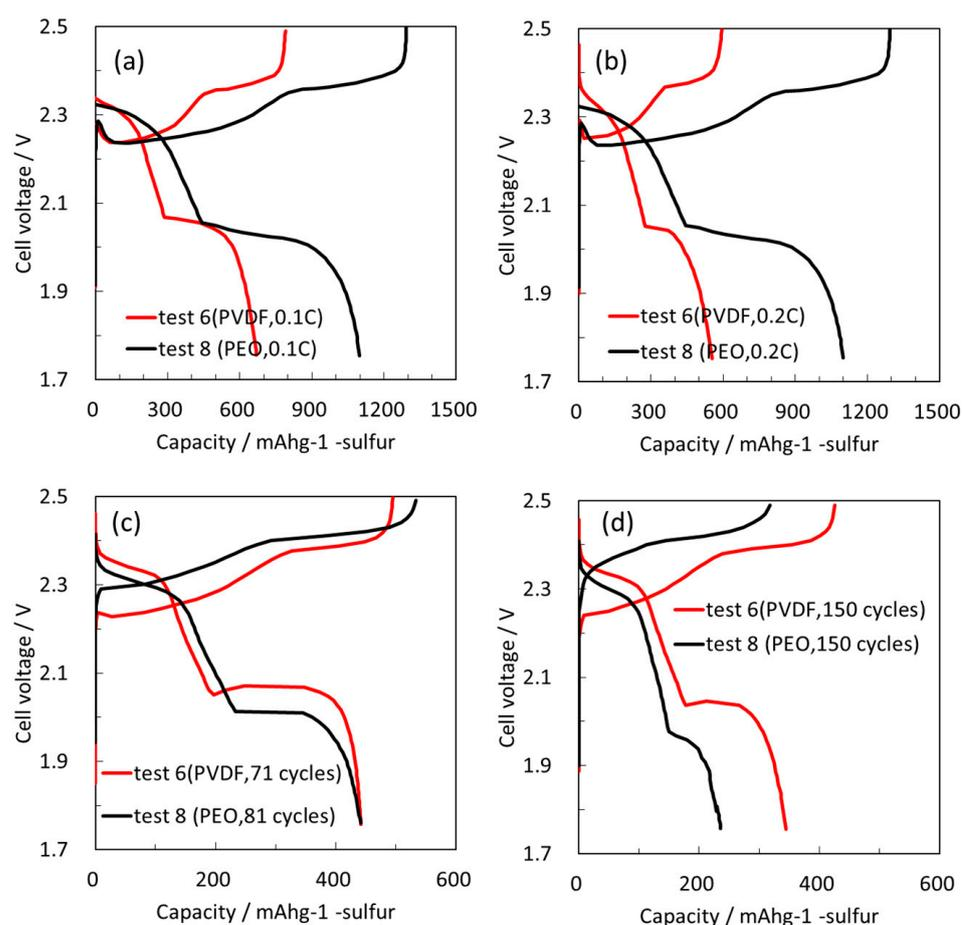
**Figure 7.** Comparison of charge/discharge voltage profiles with PEO and PVDF binders in galvanostatic cycling in standard electrolyte solutions at initial (a), second (b), 70th and 81st (same specific capacity) (c), and 150th (d) cycles. The first cycle was at 0.1 C, with further cycling at 0.2 C.
