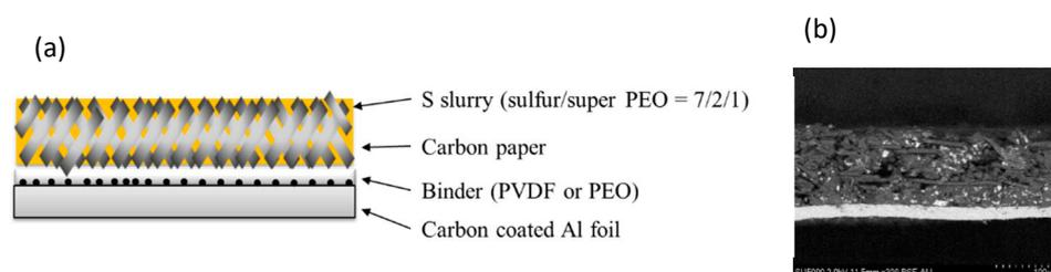
**Figure 3.** (a) Schematic image of the sulfur cathode with carbon-coated Al foil and carbon paper. (b) Cross-sectional SEM image of the electrode with S loading of 1.7 mg/cm<sup>2</sup>.
