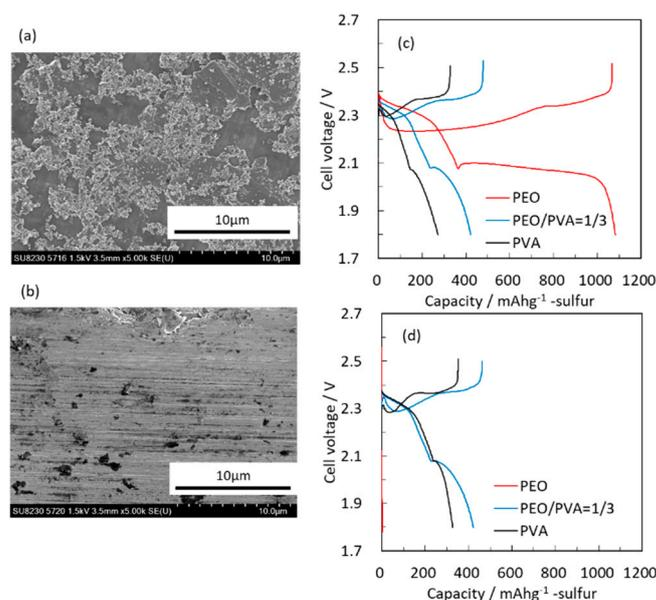
**Figure 1.** SEM images of carbon-coated (a) and glossy (b) Al current collectors and initial 0.1 C and 0.2 C charge/discharge voltage profiles in 1 M LiTFSI in 1:1 DOL/DME (c,d), respectively.
