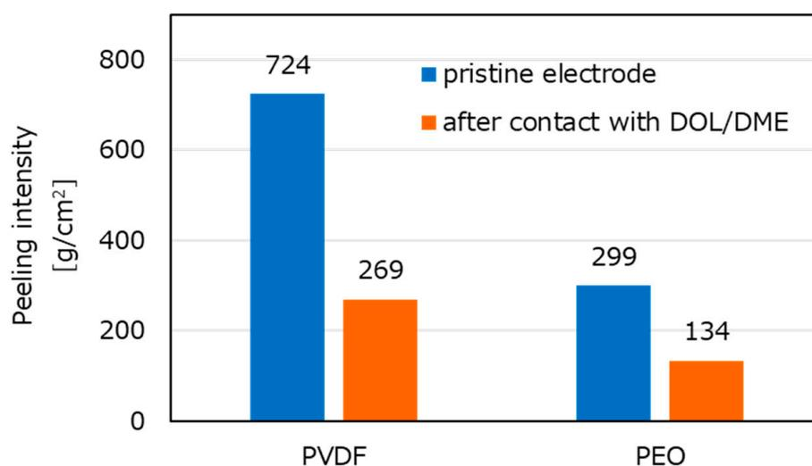
**Figure 5.** Results of peeling tests with PVDF and PEO binders for the interface between the carbon-coated Al foil and activated carbon paper before and after contact with the electrolyte solution.
