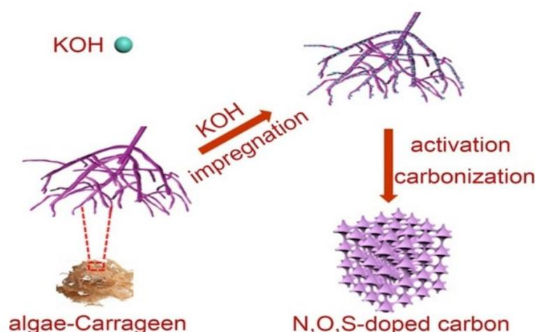
**Figure 6.** The synthesis process for the algae carrageen as hard carbon for sodium-ion batteries [51], with copyright permission from Elsevier B. V.
