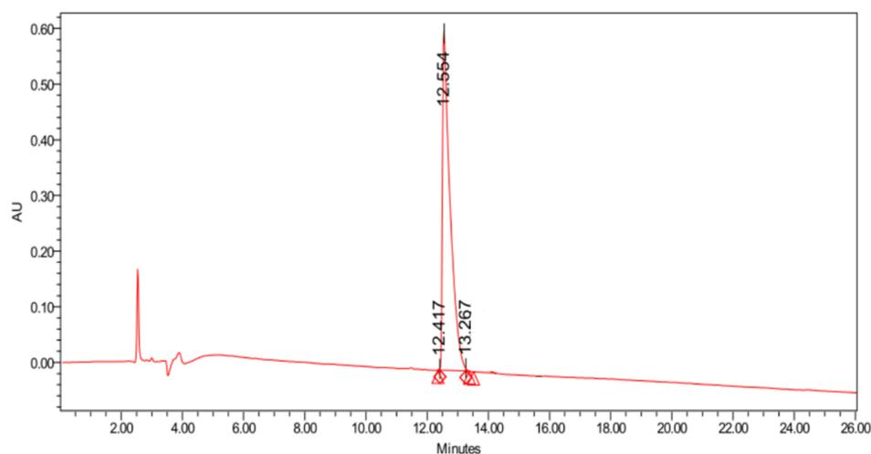
**Figure 5.** HPLC analysis of  $\text{NH}_2\text{-Ile-Thr(Bzl)-Asn-Cys(Bzl)-Pro-COOH}$  synthesized on BSA/NHS strategy.
