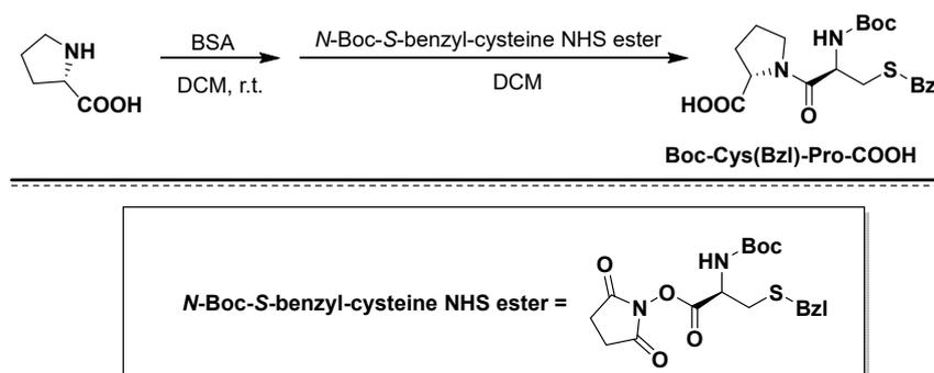
**Figure 2.** Synthesis of Boc-Cys(Bzl)-Pro-COOH using BSA/NHS as coupling agents.
