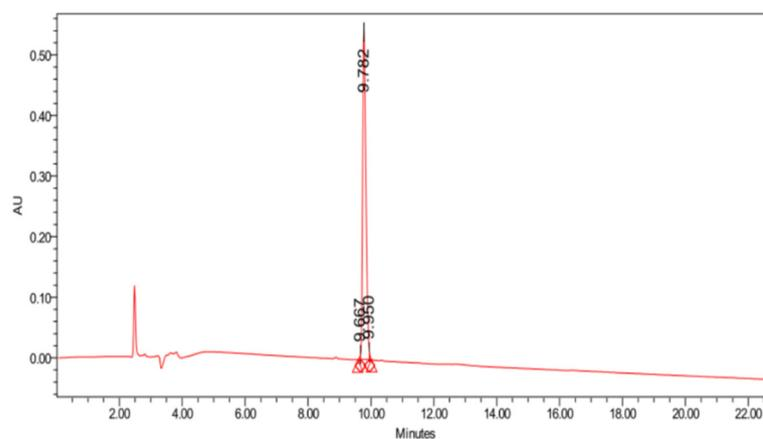
Figure 4. HPLC analysis of NH<sub>2</sub>-Cys(Bzl)-Pro-COOH.
