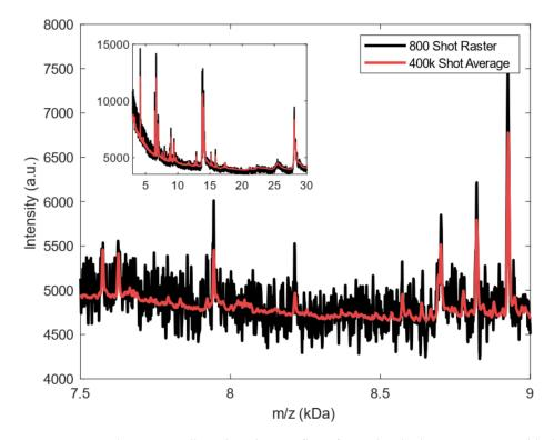
**Figure 1.** Example spectra collected on the RapifleX of an individual raster spectrum (black) and a 400,000 shot Deep MALDI averaged spectrum (red) from 7.5 to 9 kDa m/z range. The inset shows the same spectra over the full 3 to 30 kDa range analyzed in this work.
