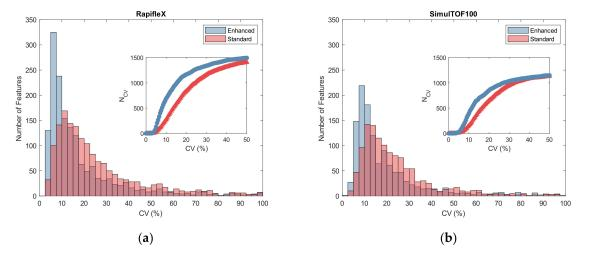
**Figure 6.** Reproducibility of feature values for a single sample over 20 preparations and acquisitions collected on the (**a**) RapifleX and (**b**) SimulTOF100. Histograms of CVs for standard (red) and enhanced (blue) feature values are shown in the main plot. The inset shows the cumulative CV distribution,  $N_{CV}$ , for the standard (red, triangles) and enhanced feature values (blue, circles) (only CVs up to 50% are shown for clarity).
