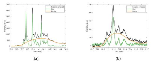
**Figure 2.** Spectral component analysis showing the baseline corrected Deep MALDI spectrum (black), fine structure (green), and bumps (orange) for peak clusters around (**a**) 14 kDa and (**b**) 21 kDa.
