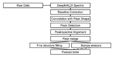
**Scheme 1.** Spectral analysis workflow for mass spectrometer data using presented preprocessing methods.
