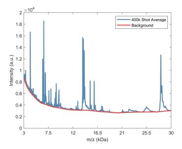
**Figure 4.** Example of a 400,000 shot-averaged Deep MALDI spectrum collected on the RapifleX and the associated Eilers' background estimation.
