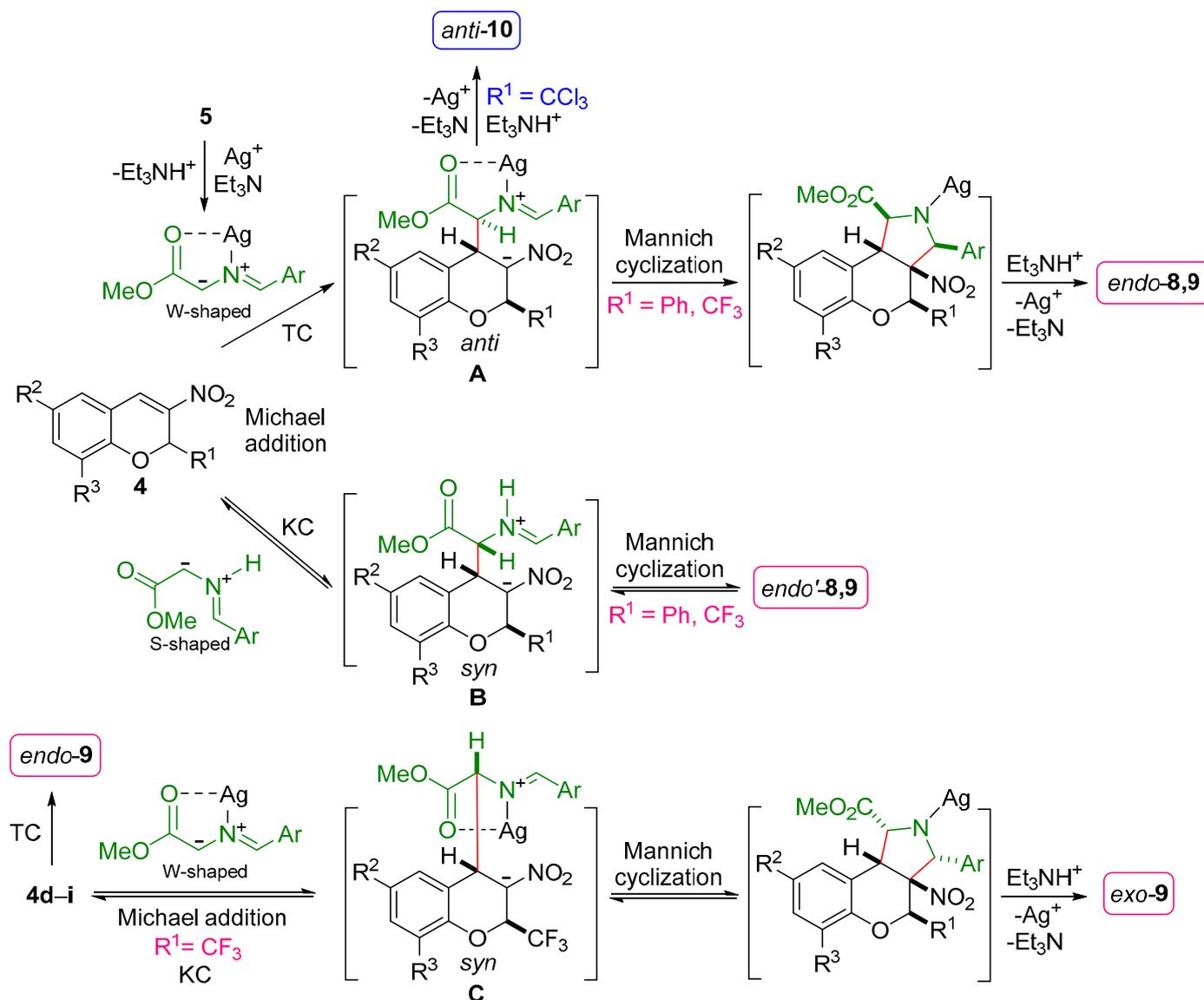
**Scheme 8.** Proposed mechanism for the AgOAc-catalyzed reaction of chromenes 4 with iminoesters 5.
