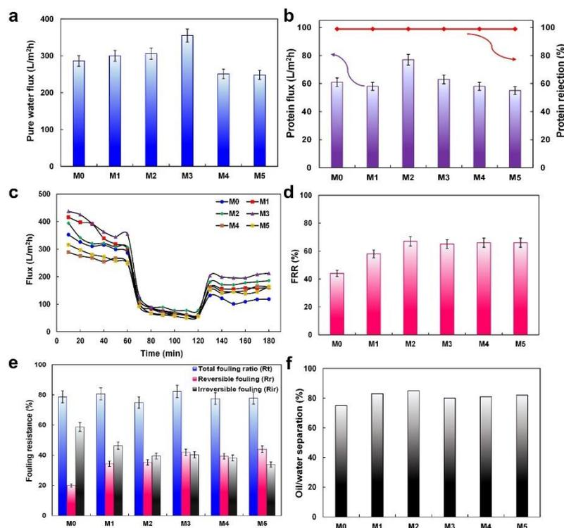
**Figure 5.** (a) The PWF, (b) flux and rejection of protein, (c) membrane flux against time. “The 1st, 2nd, and 3rd 60 min illustrate the PWF, protein solution flux, and the PWF after membrane cleaning, respectively”. (d) FRR%, (e) fouling ratio parameters, and (f) oil/water separation of different membranes.
