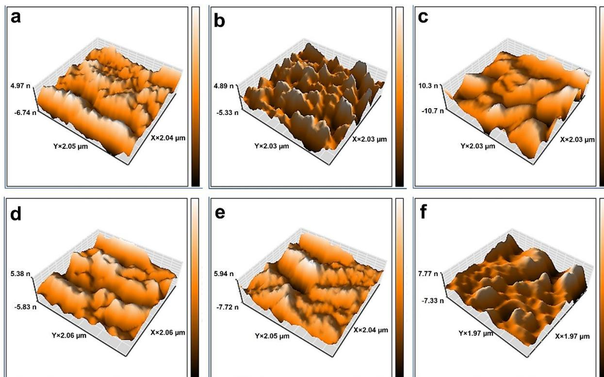
**Figure 4.** AFM topographical illustrations of various membranes: (a) M0, (b) M1, (c) M2, (d) M3, (e) M4, and (f) M5.
