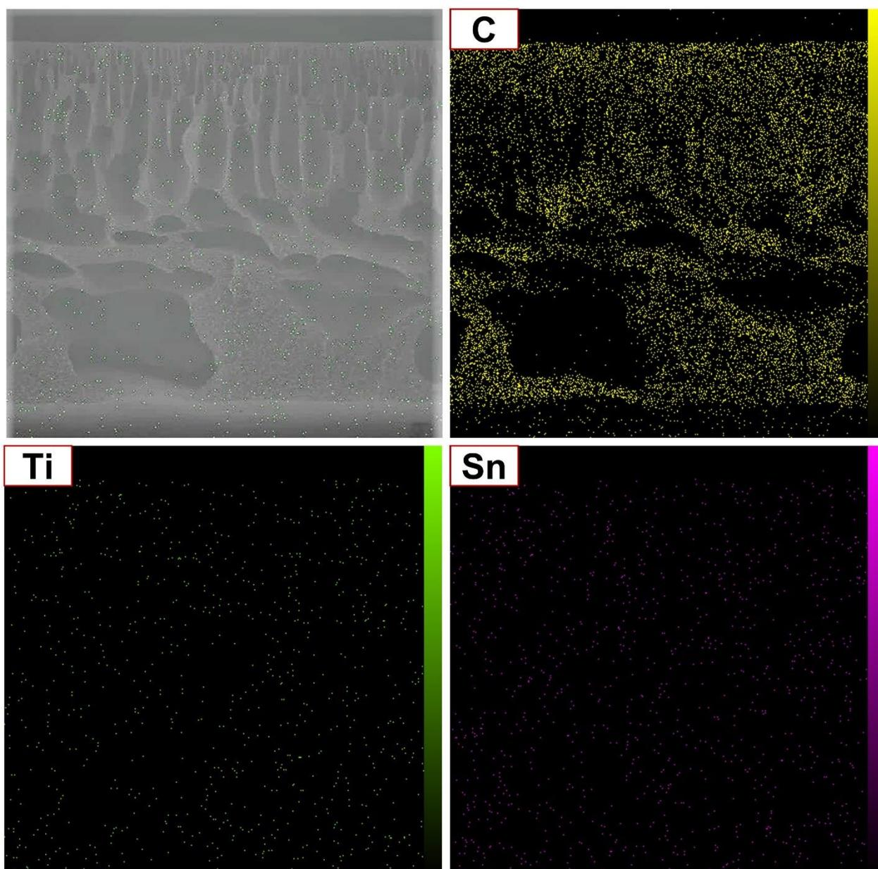
**Figure 3.** EDAX dot mapping analysis of M3 membrane sample.
