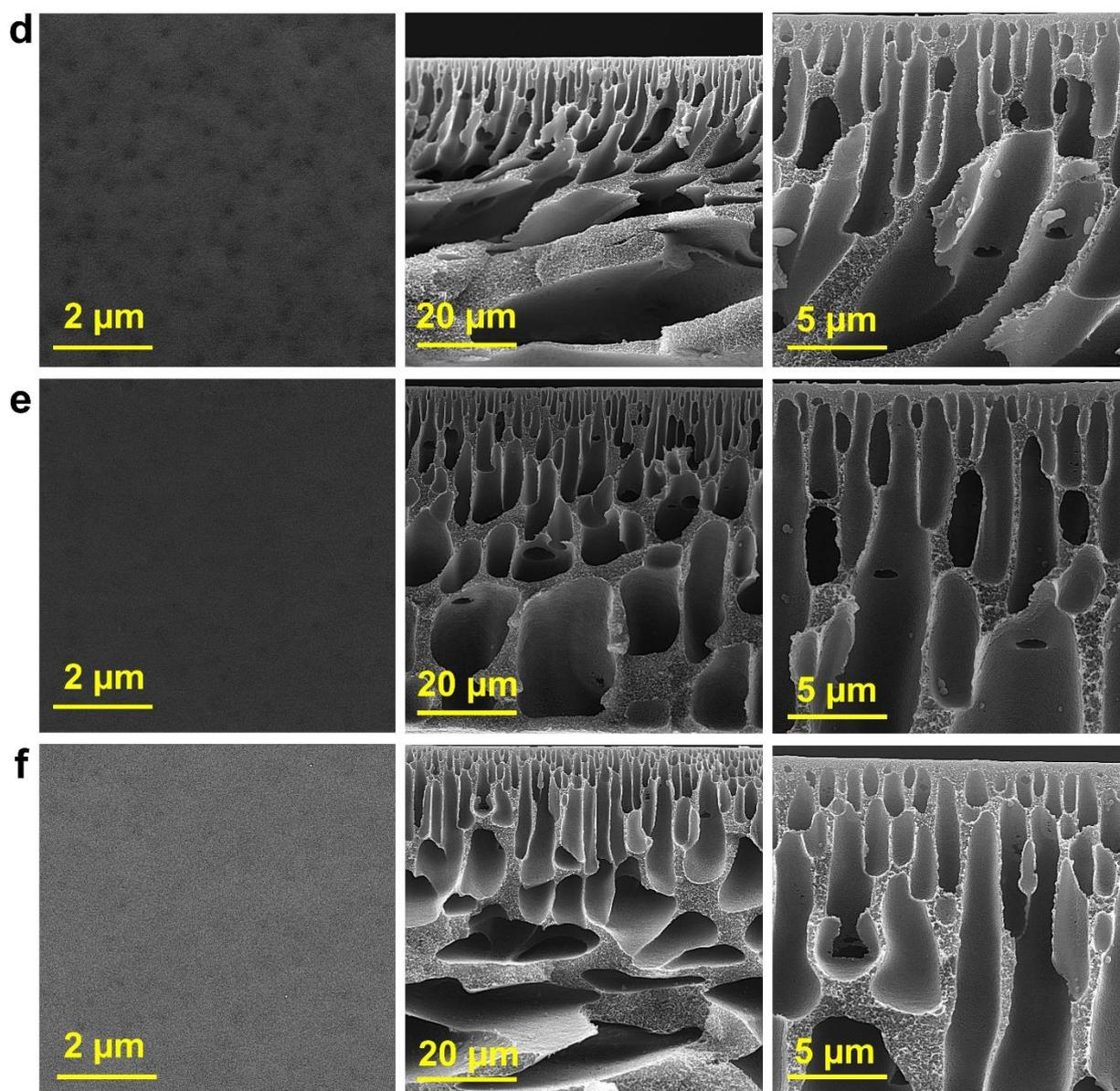
**Figure 2.** SEM micrographs from surface and cross-sections of various membranes at three different scales of 2, 5, and 20  $\mu\text{m}$ : (a) M0, (b) M1, (c) M2, (d) M3, (e) M4, and (f) M5.
