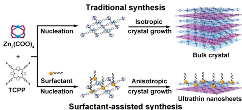
**Figure 10.** The traditional synthesis and surfactant-assisted synthesis of MOFs. Top: During the synthesis of MOFs in the traditional method, the isotropic growth generates the bulk crystal of MOFs. Bottom: By using developed surfactant-assisted synthetic method, resulting in the formation of ultrathin MOFs nanosheets. Reprinted from [69] with permission from Wiley.
