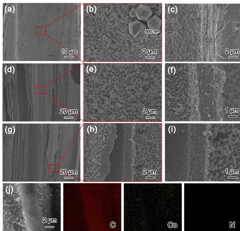
**Figure 2.** SEM images of HZ@Wood (a–c), Zn-Co@CW (d–f), and Zn-Co<sub>3</sub>O<sub>4</sub>@CW-230 (g–i); C, Co, Zn mapping of Zn-Co<sub>3</sub>O<sub>4</sub>@CW-230 (j).
