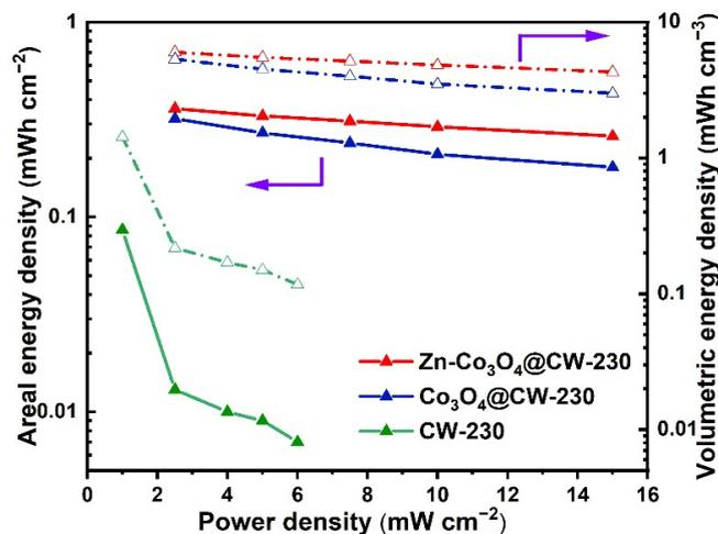
**Figure 6.** Areal energy density and volumetric energy density at different power densities of the SC of CW-230, Co<sub>3</sub>O<sub>4</sub>@CW-230, and Zn-Co<sub>3</sub>O<sub>4</sub>@CW-230.
