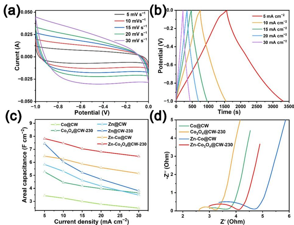
**Figure 4.** Cyclic voltammograms (CVs) at different scan rates and galvanostatic charge-discharge (GCD) curves at different current densities of (a,b) Zn-Co<sub>3</sub>O<sub>4</sub>@CW-230. (c) Specific capacitances of Zn/Co/Zn-Co@CW and Zn/Co<sub>3</sub>O<sub>4</sub>/Zn-Co<sub>3</sub>O<sub>4</sub>@CW-230 at different current densities. (d) the EIS plots of the Co/Zn-Co@CW and Co<sub>3</sub>O<sub>4</sub>/Zn-Co<sub>3</sub>O<sub>4</sub>@CW-230.
