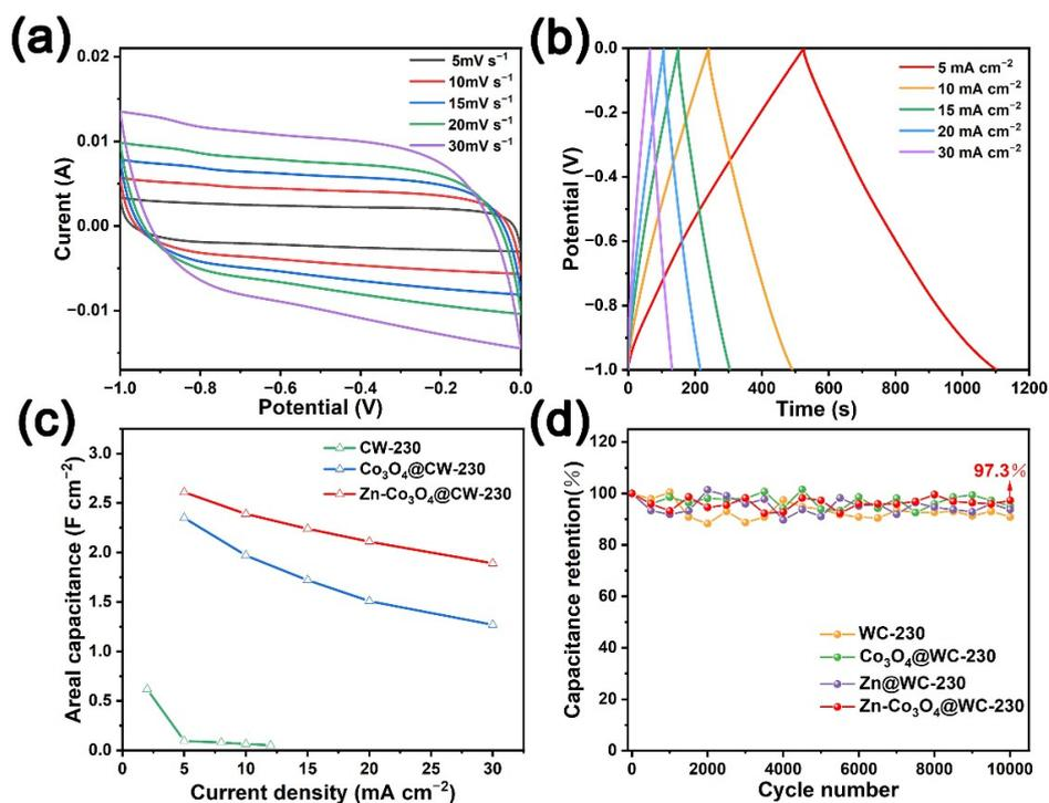
**Figure 5.** Capacitive performance of the SC of Zn-Co<sub>3</sub>O<sub>4</sub>@CW-230: (a) cyclic voltammograms at various scan rates in a two-electrode system, and (b) GCD profiles at different current densities. (c) Rate performances based on the GCD curves at different current densities, (d) the SC device measured at 50 mA cm<sup>-2</sup> for 10,000 cycles.
