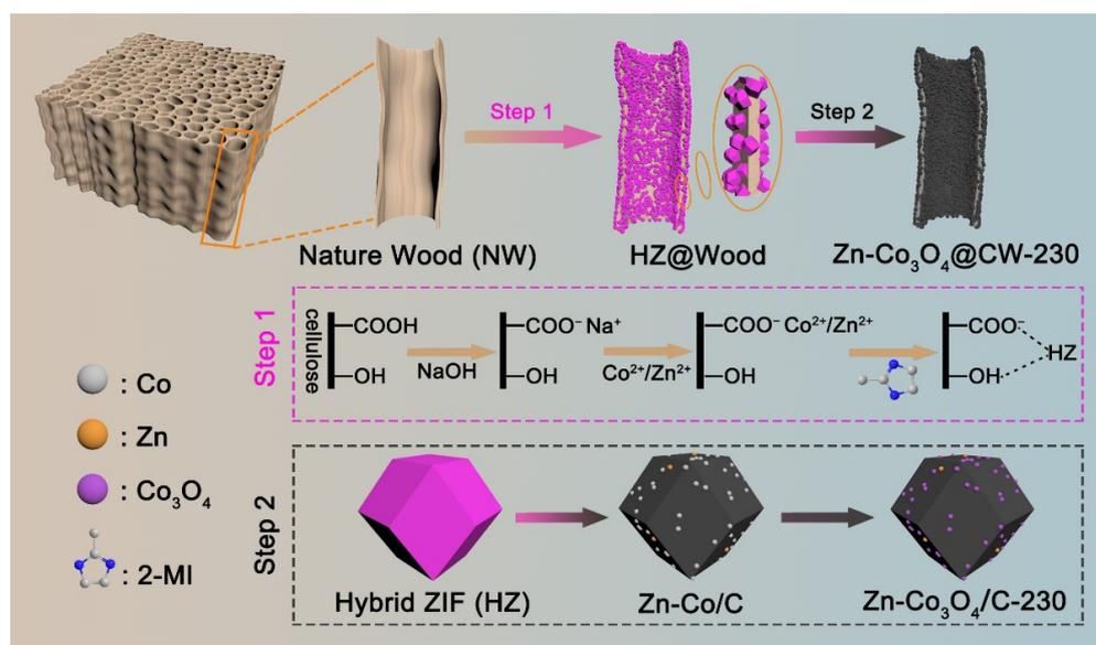
**Figure 1.** Schematic representation of the fabrication procedure for Zn-Co<sub>3</sub>O<sub>4</sub>@CW-230.
