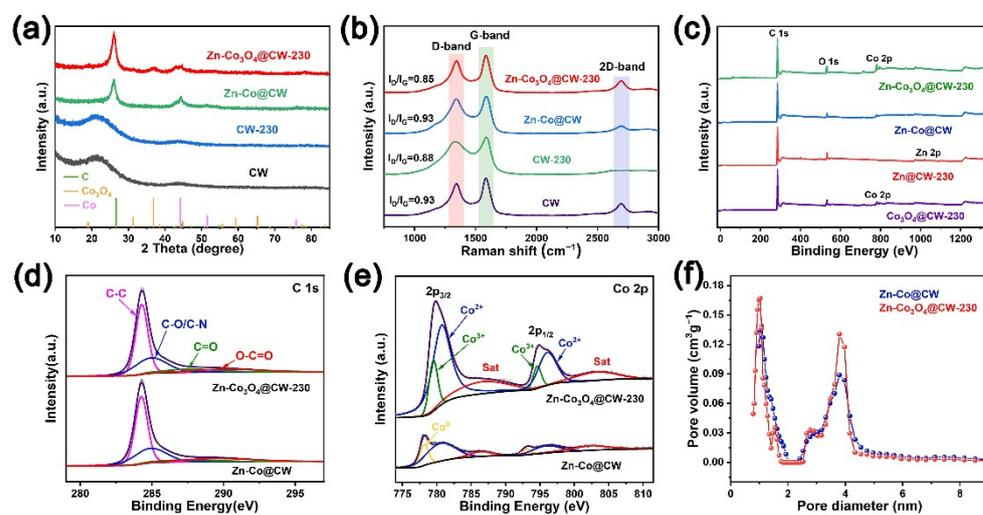
**Figure 3.** (a) XRD spectra of CW, CW-230, Zn-Co@CW, and Zn- $\text{Co}_3\text{O}_4$ @CW-230; and Raman spectra (b). XPS spectra of (c) full scan survey for  $\text{Co}_3\text{O}_4$ @CW-230, Zn@CW-230, Zn-Co@CW, and Zn- $\text{Co}_3\text{O}_4$ @CW-230. High-resolution XPS spectra of Zn-Co@CW and Zn- $\text{Co}_3\text{O}_4$ @CW-230 for (d) C 1s and (e) Co 2p; and (f) corresponding pore size distribution.
