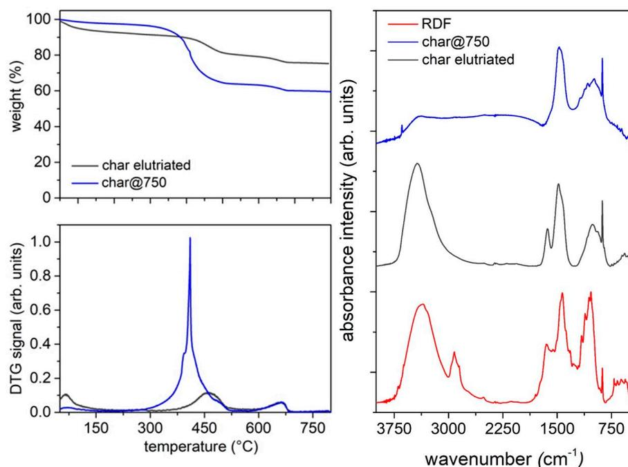
**Figure 11.** Left panels: TG curves (up) and the corresponding DTG curves (down) of the elutriated char and char@750 (oxidizing atmosphere, air); right panel: FTIR spectra of RDF, elutriated char and char@750.
