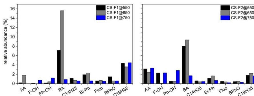
**Figure 7.** Comparison of the abundances of selected species present in CS mixtures collected in flask 1 and flask 2 after RDF pyrolysis tests up to 550, 650 and 750 °C (acetic acid (AA), 2-furan methanol (F-OH), phenol (Ph-OH), benzoic acid (BA), tetradecane (C<sub>14</sub>H<sub>28</sub>), biphenyl (Bi-Ph), fluorene (Fluo), benzophenone (BPhO) and 1-nonadecene (C<sub>19</sub>H<sub>38</sub>)).
