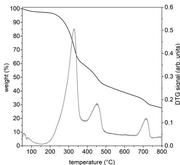
**Figure 1.** Thermogravimetric curve of RDF at 30 °C/min, N<sub>2</sub> atmosphere (black line) and the corresponding derivative (DTG) curve (grey line).
