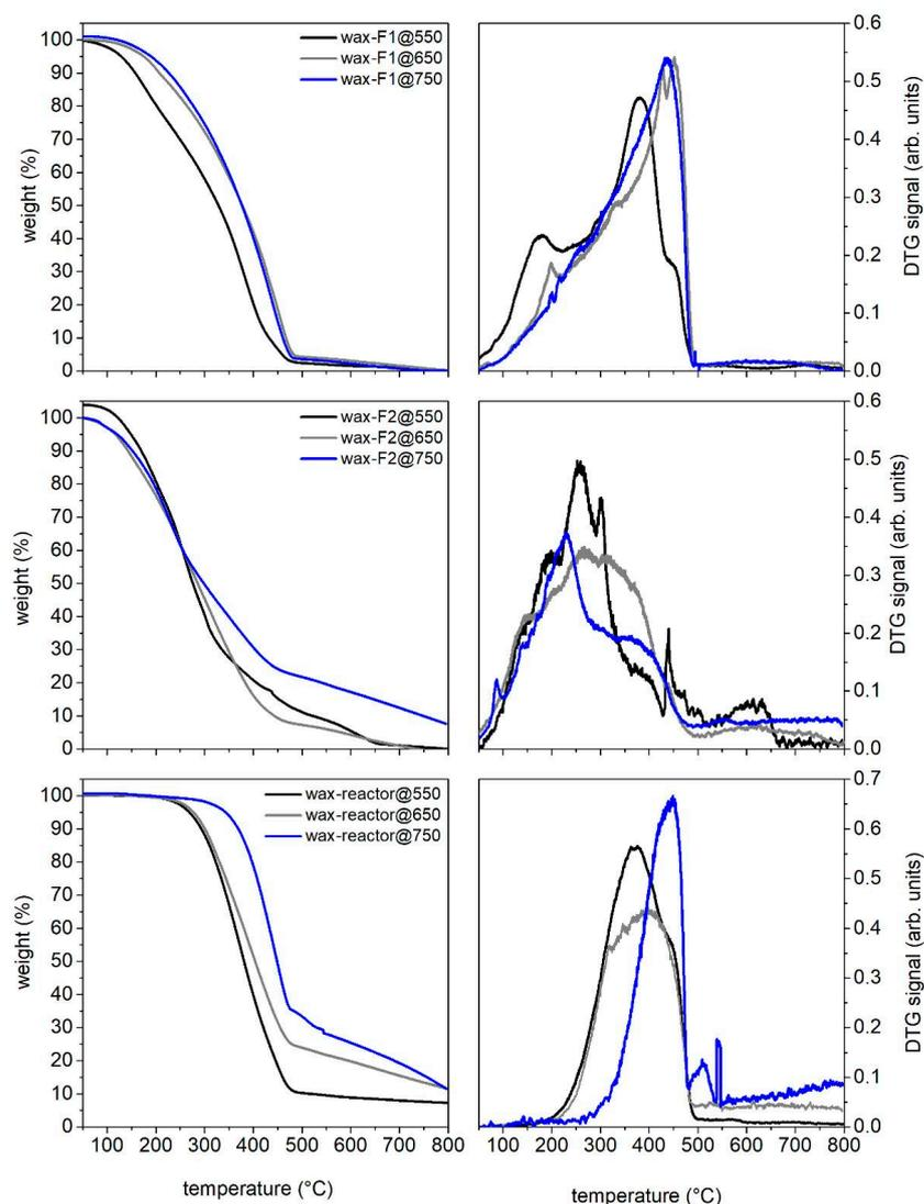
**Figure 8.** TG profiles and the corresponding DTG curves of waxy solids recovered after RDF pyrolysis tests up to 550, 650 and 750 °C. TG analyses have been performed under nitrogen atmosphere (flux 40 mL/min, HR 10 °C/min).
