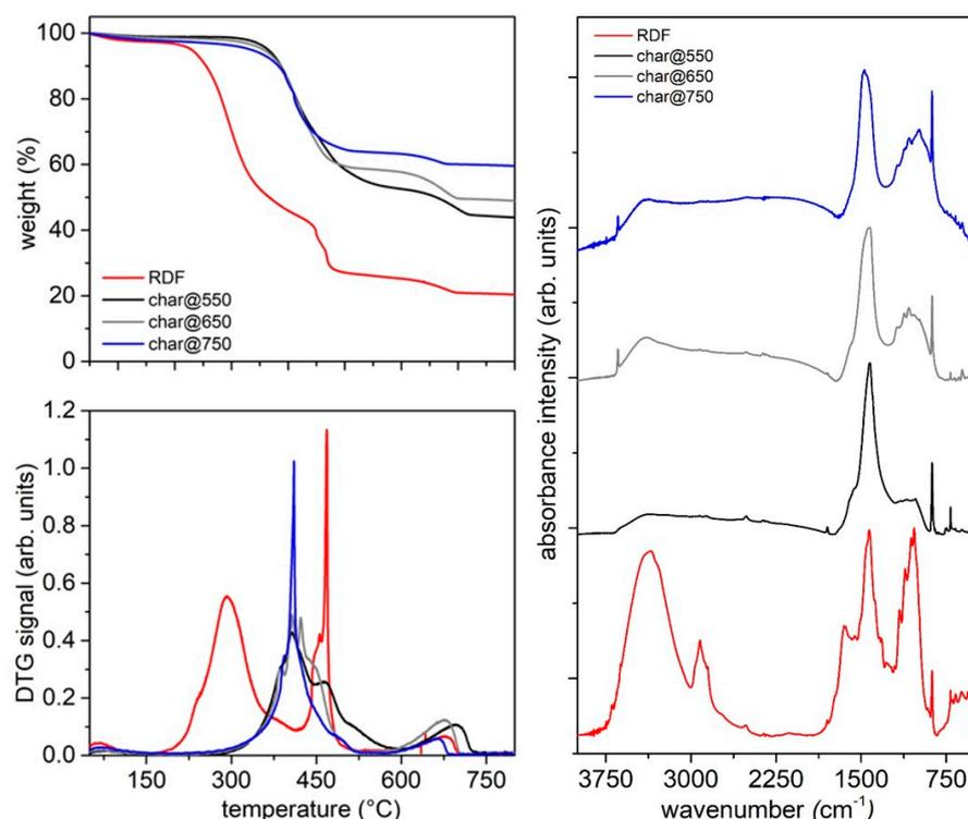
**Figure 5.** Left panels: TG profiles (up) and DTG curves (down) of char samples and RDF in oxidative atmosphere (synthetic air, flux 40 mL/min, HR 10 °C/min); right panel: height-normalized FTIR spectra of RDF, char@550, char@650 and char@750.
