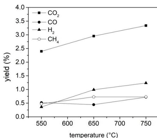
**Figure 3.** Yields of H<sub>2</sub>, CO, CO<sub>2</sub> and CH<sub>4</sub> as a function of the final pyrolysis temperature.
