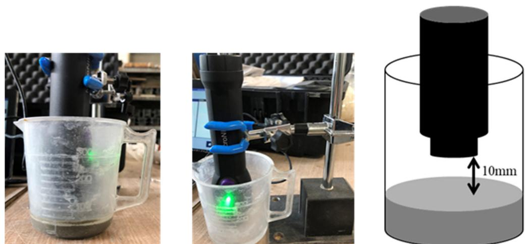
**Figure 14.** Spectral measurement immediately after mixing (cement paste).
