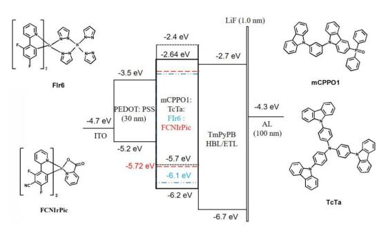
**Figure 1.** Energy levels diagram of the blue PhOLEDs and molecular structures used in this work, FIr6 (blue dash dot line), FCNIrPic (red dashed line).
