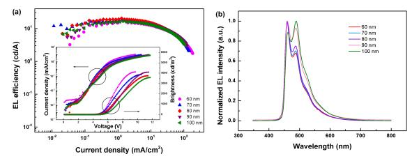
**Figure 5.** (a) EL efficiency-current density ( $\eta$ -*J*) characteristics of co-dopant devices with ETL at different thicknesses. Inset: Current density-brightness-voltage (*J*-*B*-*V*) characteristics of co-dopant devices with ETL at different thicknesses. (b) Normalized EL spectra of devices with ETL at different thicknesses operating at the current density of 10 mA/cm<sup>2</sup>.
