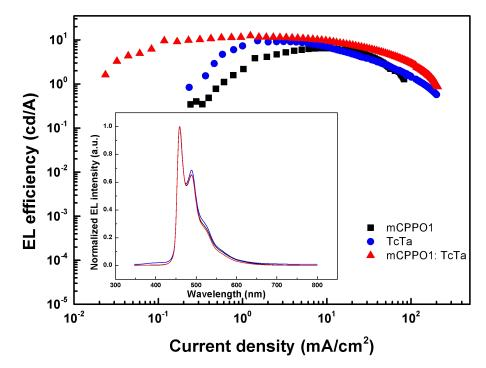
**Figure 2.** EL efficiency-current density ( $\eta$ -*J*) characteristics of devices with FIr6 doped into different hosts. Inset: Normalized EL spectra of devices with FIr6 doped into different hosts operating at 10 mA/cm<sup>2</sup>.
