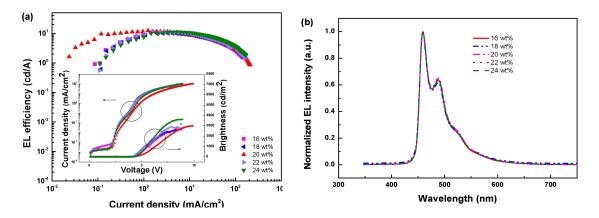
**Figure 3.** (a) EL efficiency-current density ( $\eta$ -*J*) characteristics of co-host devices with FIr6 at different doping concentrations. Inset: Current density-brightness-voltage (*J*-*B*-*V*) characteristics of co-host devices with FIr6 at different doping concentrations. (b) Normalized EL spectra of co-host devices with FIr6 at different doping concentrations operating at the current density of 10 mA/cm<sup>2</sup>.
