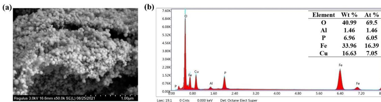
Figure 1. SEM image (a) and EDS spectroscopy (b) of  $\text{CuFe}_2\text{O}_4$ .
