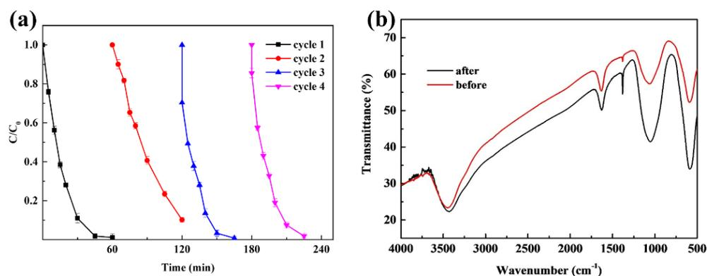
**Figure 8.** (a) Reusability of  $\text{CuFe}_2\text{O}_4$  (PAA = 80 mg/L,  $\text{CuFe}_2\text{O}_4$  = 100 mg/L, pH = 7,  $C_0$  = 20 mg/L, room temperature for 1 h). (b) FTIR spectra of  $\text{CuFe}_2\text{O}_4$ .
