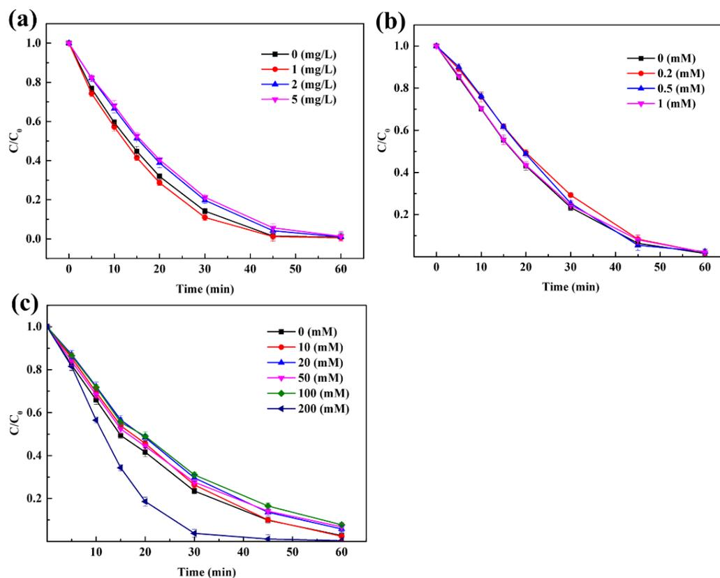
**Figure 7.** Effect of water matrices. (a) HA. (b)  $\text{HCO}_3^-$ . (c)  $\text{Cl}^-$  (PAA = 80 mg/L,  $\text{CuFe}_2\text{O}_4$  = 100 mg/L, pH = 7,  $C_0$  = 20 mg/L, room temperature for 1 h).
