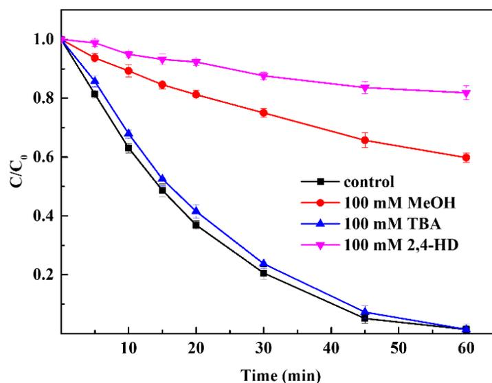
**Figure 5.** Effect of radical scavengers on Rhodamine B degradation (PAA = 80 mg/L,  $\text{CuFe}_2\text{O}_4$  = 100 mg/L, pH = 7,  $C_0$  = 20 mg/L, room temperature for 1 h).
