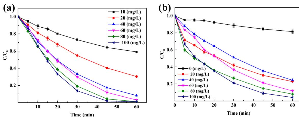
**Figure 3.** (a) Effect of PAA loading on Rhodamine B degradation ( $\text{CuFe}_2\text{O}_4 = 100$  mg/L, pH = 7,  $C_0 = 20$  mg/L, room temperature for 1 h). (b) Effect of catalyst loading on Rhodamine B degradation (PAA = 80 mg/L, pH = 7,  $C_0 = 20$  mg/L, room temperature for 1 h).
