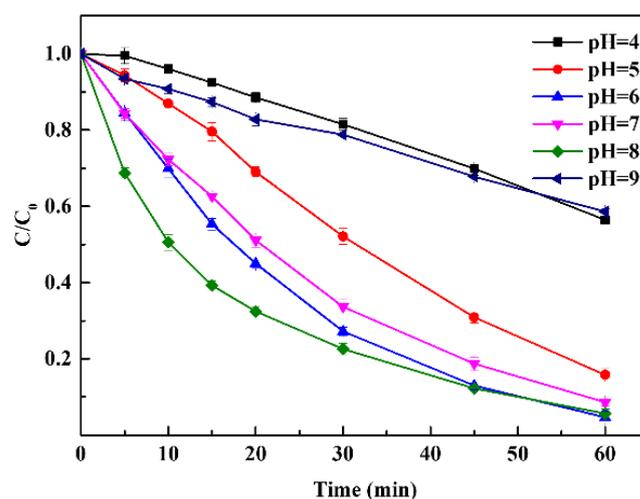
**Figure 2.** Effect of pH on Rhodamine B degradation ( $\text{CuFe}_2\text{O}_4 = 100$  mg/L, PAA = 40 mg/L,  $C_0 = 20$  mg/L, room temperature for 1 h).
