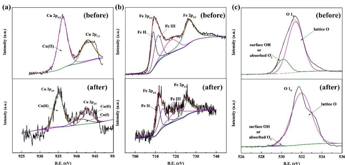
**Figure 4.** XPS spectra of  $\text{CuFe}_2\text{O}_4$ . (a) Cu. (b) Fe. (c) O.
