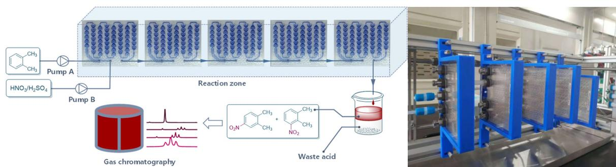
**Figure 2.** Continuous-flow reactor setup for condition optimization.
