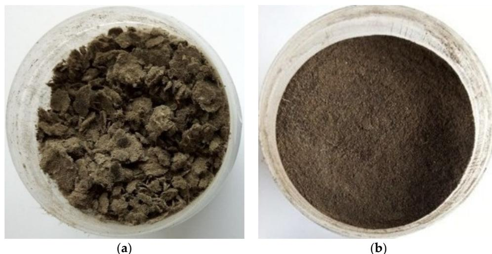
**Figure 1.** The (a) primary and (b) dewatered sludge after grinding and/or sieving.
