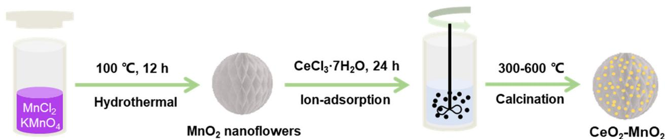
**Scheme 1.** Schematic of the synthesis process for  $\text{CeO}_2\text{-MnO}_2$  nanocomposites.
