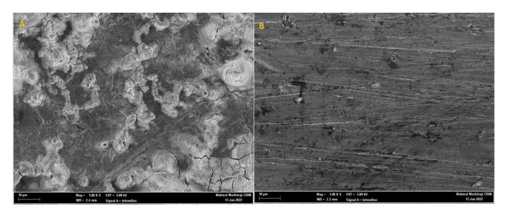
**Figure 10.** SEM micrographs showing the surface morphology of mild-steel-coupon surface in absence (**A**) and presence (**B**) of 0.0005 M PMBMH in 1 M HCl environment for 5 h at 303 K.
