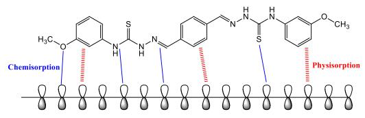
**Figure 12.** Suggested corrosion-inhibition mechanism of mild steel in 1 M HCl with the addition of the examined inhibitor.
