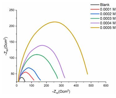
**Figure 8.** Nyquist plots of mild steel in 1 M HCl without and with the addition of various concentrations of PMBMH.
