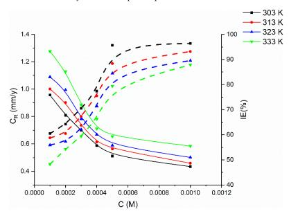
**Figure 3.** Gravimetric-curve relationship of metal coupons in 1 M HCl between corrosion rate and inhibition efficiency against concentration of PMBMH at different temperatures for 5 h exposure period.
