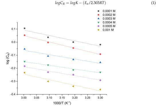
Arrhenius Equation (1) was used to calculate the activation parameters of the corrosion process (Figure 4):
