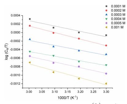
**Figure 5.** A plot of Arrhenius modified equations of  $log\left\{\frac{C_R}{T}\right\}$  versus  $\frac{i}{T}$  for tested metal with different concentrations of the examined inhibitor.
