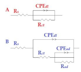
**Figure 9.** The model of equivalent circuit that was used to fit the experimental data (**A**) without and (**B**) with the addition of the tested inhibitor.
