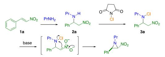
Scheme 1. A mechanism for the formation of nitroaziridine from  $\beta$ -nitrostyrene 1a.
