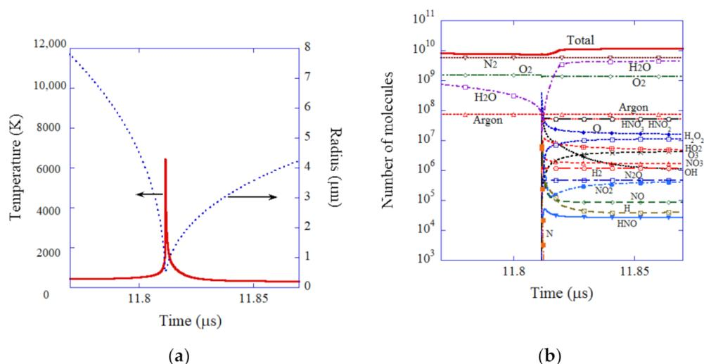
**Figure 4.** The results of the numerical simulation for an initial air bubble as a function of time at around the end of the violent bubble collapse for 0.1 μs [40]. (a) The bubble radius and the temperature inside a bubble. (b) The number of molecules inside a bubble. Copyright 2005, with permission of AIP Publishing.
