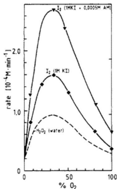
**Figure 11.** Experimental results on the rate of production of  $\text{H}_2\text{O}_2$  in pure water and that of  $\text{I}_2$  in 1 M KI solution or 1 M KI + 0.0005 M ammonium molybdate solution under various mixtures of argon and oxygen dissolved in the solution irradiated with ultrasound of 300 kHz [122]. Copyright 1985, with permission from the American Chemical Society.
