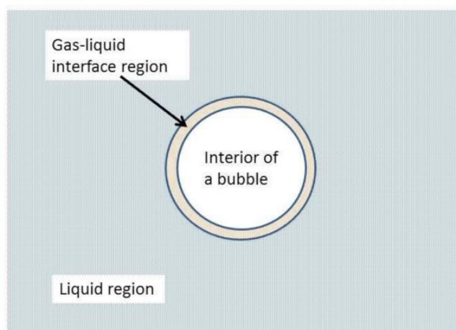
**Figure 10.** Three regions for a cavitation bubble [109]. Copyright 2016, with permission from Springer.
