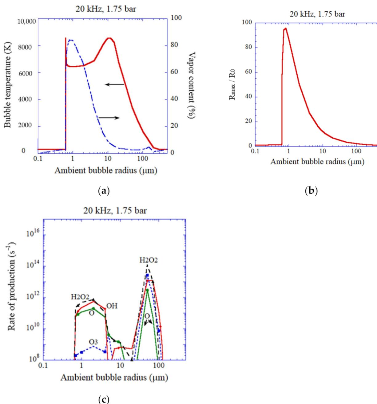
**Figure 7.** The results of the numerical simulations as a function of ambient bubble radius for an isolated air bubble when frequency and pressure amplitude of ultrasound are 20 kHz and 1.75 bar, respectively [59]. (a) The temperature inside a bubble and the molar fraction of water vapor at the violent collapse. (b) The expansion ratio. (c) The rate of production of each oxidant. Copyright 2008, with permission of AIP Publishing.
