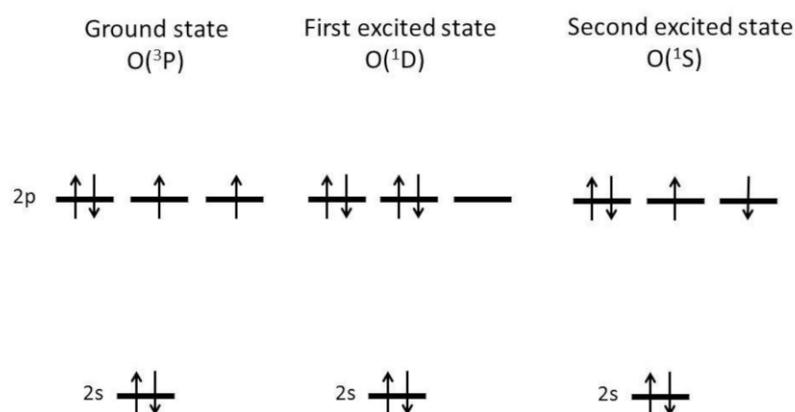
**Figure 9.** Electronic configurations of ground state, first excited state, and second excited state of the oxygen atom [109]. Two electrons in the 1s state are omitted. Copyright 2016, with permission from Springer.
