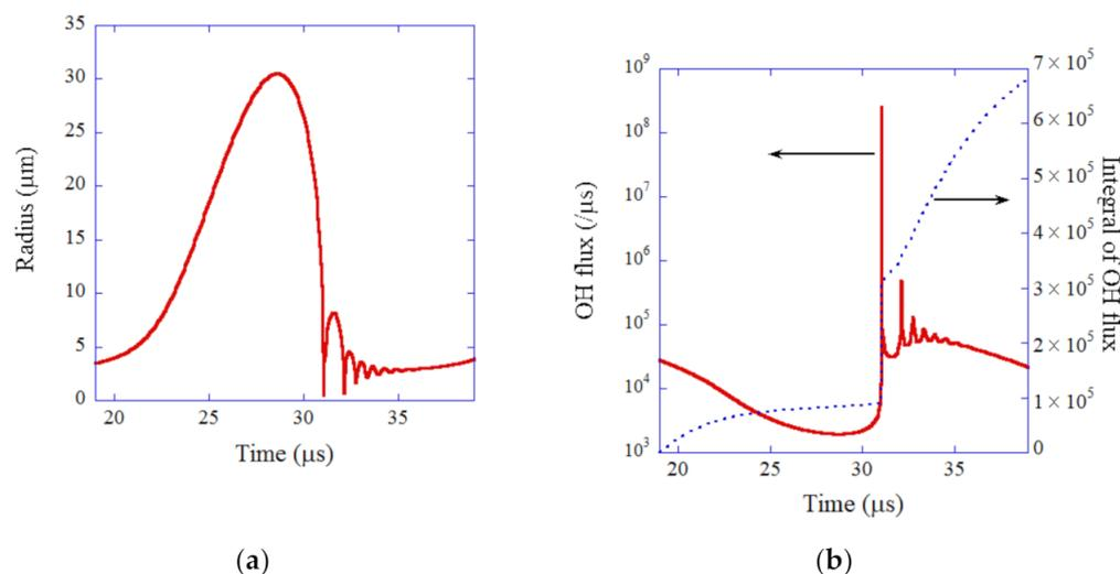
**Figure 2.** The results of the numerical simulation under the experimental condition of single-bubble sonochemistry as a function of time for one acoustic cycle [40]. The frequency and pressure amplitude of ultrasound are 52 kHz and 1.52 bar, respectively. (a) The bubble radius. (b) The dissolution rate of OH radicals into the liquid from the interior of the bubble (red solid line) and its time integral (blue dotted line). Copyright 2005, with permission of AIP Publishing.
