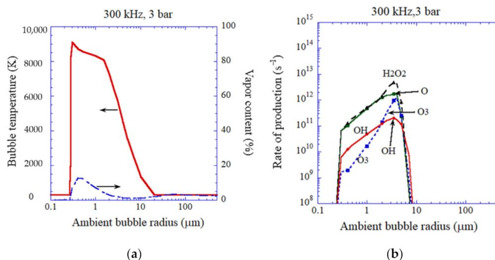
**Figure 8.** The results of the numerical simulations as a function of ambient bubble radius for an isolated air bubble for 300 kHz and 3 bar [59]. (a) The temperature inside a bubble and the molar fraction of water vapor at the violent collapse. (b) The rate of production of each oxidant. Copyright 2008, with permission of AIP Publishing.
