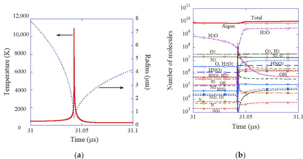
**Figure 3.** The results of the numerical simulations for an argon bubble under the condition of Figure 2 as a function of time at approximately the end of the violent bubble collapse for 0.1 μs [40]. (a) The bubble radius and the temperature inside a bubble. (b) The number of molecules inside a bubble. Copyright 2005, with permission of AIP Publishing.
