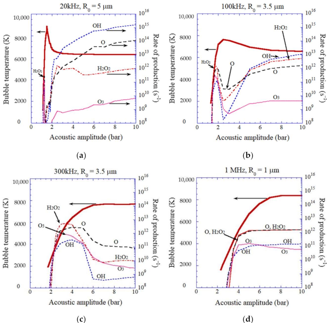
**Figure 6.** The results of the numerical simulations on the rate of production of each oxidant inside an isolated air bubble calculated by the first bubble collapse as a function of acoustic amplitude as well as the temperature inside a bubble at the end of the bubble collapse (the red thick line) [41]. (a) 20 kHz, (b) 100 kHz, (c) 300 kHz, (d) 1 MHz. Copyright 2007, with permission of AIP Publishing.
