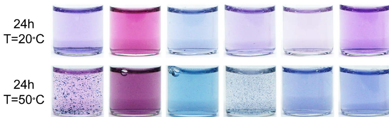
Figure S31. The colour change of mixture solutions containing Pd(II), tropaeolin and other metal cations: \text{Zn}^{2+} , \text{Ni}^{2+} , \text{Mg}^{2+} , \text{K}^+ , \text{Co}^{2+} , \text{Al}^{3+} , after 5min, 1h and 24h in temperature 20^\circ\text{C} and 50^\circ\text{C} . Conditions: C_{0,\text{TR}} = 1,875 \cdot 10^{-5} \text{ mol/dm}^3 , C_{0,\text{Pd(II)}} = 3,125 \cdot 10^{-5} \text{ mol/dm}^3 , C_{0,\text{anions}} = 0.0625 \text{ mol/dm}^3 , volumetric ratio mixing Pd(II) ions and tropaeolin 2.5mL: 1.5mL, pH = 4.10.
