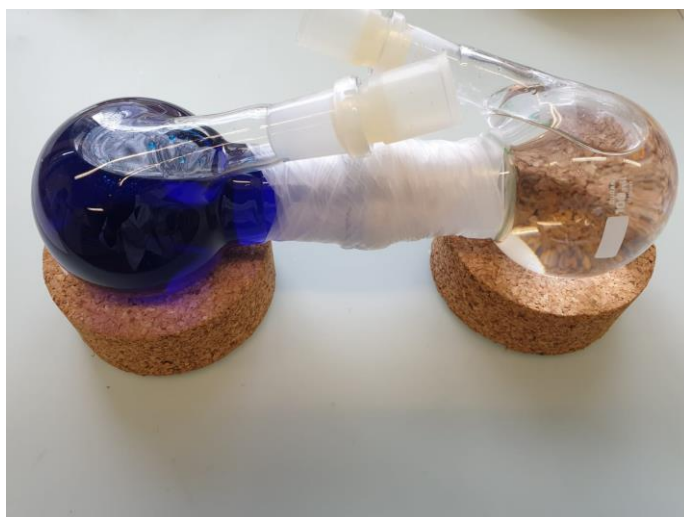
Figure S5. Photo of the “home-built” diffusion cell for testing the V(IV) diffusion through the membranes (NR212, FAP-450 and PP-PBI).
