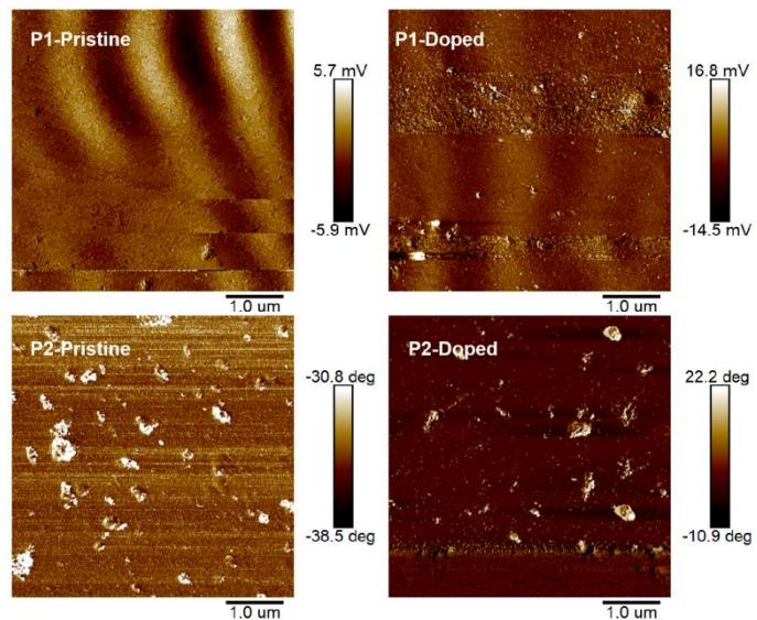
**Figure S8.** AFM phase images of P1 and P2 before and after doping.
