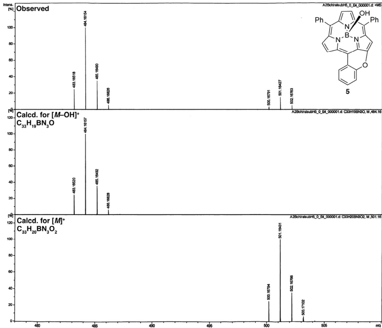
**Figure S2.** High-resolution mass spectrum of **5**, observed spectrum (top) and isotopic patterns calculated for C<sub>33</sub>H<sub>19</sub>BN<sub>3</sub>O as a [M-OH]<sup>+</sup> ion (middle) and C<sub>33</sub>H<sub>20</sub>BN<sub>3</sub>O<sub>2</sub> as a [M]<sup>+</sup> ion (bottom).
