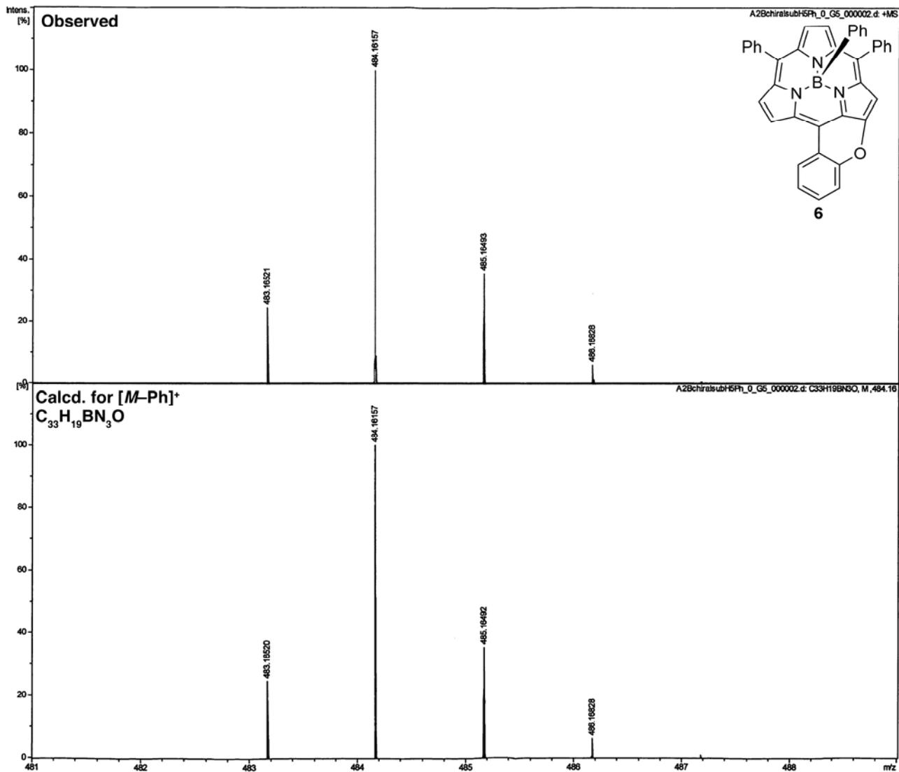
**Figure S3.** High-resolution mass spectrum of **6**, observed spectrum (top) and isotopic patterns calculated for  $C_{33}H_{19}BN_3O$  as a  $[M-Ph]^+$  ion (bottom).
