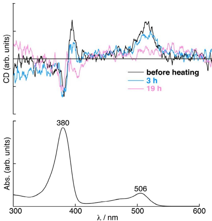
**Figure S6.** CD (top) and UV/vis absorption (bottom) spectra of 5 in CH<sub>2</sub>Cl<sub>2</sub> after chiral resolution (black line) and after heating at 40 °C for 3 h (aqua blue line) and 19 h (pink line).
