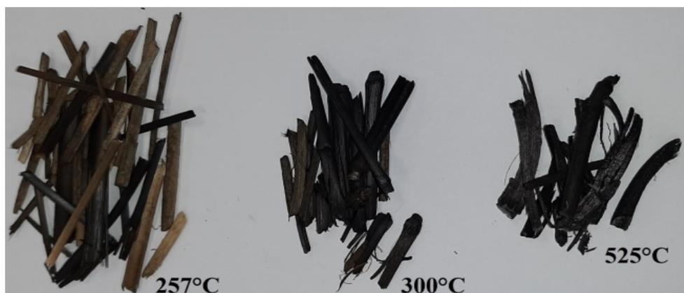
**Figure 20.** Torrefied Miscanthus samples after process at selected temperatures.
