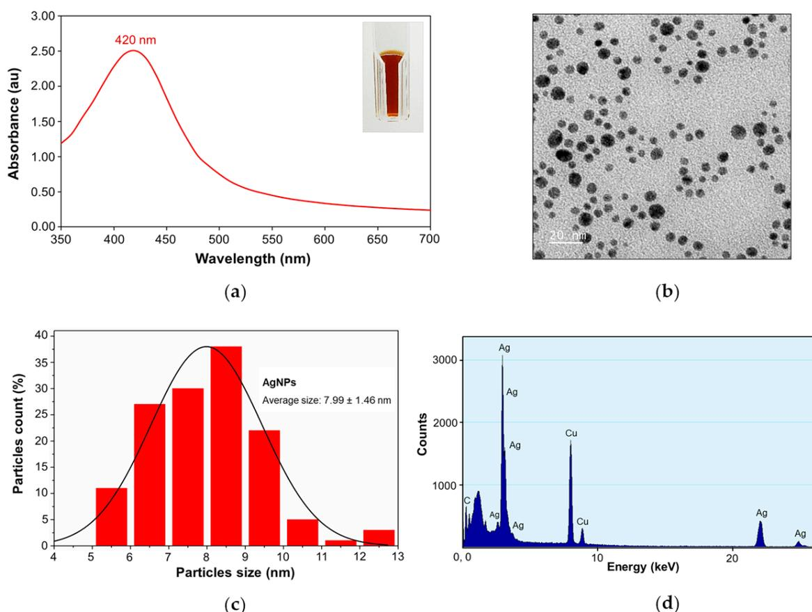
**Figure 1.** Physicochemical characterization of silver nanoparticles: (a) UV-Vis spectra of silver nanoparticles at 420 nm, inset: the dark yellow color of AgNPs; (b) transmission electron micrograph (TEM) of AgNPs showing the NPs spherical shape; (c) the average size of  $7.99 \pm 1.46$  nm ( $n = 137$ ); (d) and the EDX spectrum of AgNPs.
