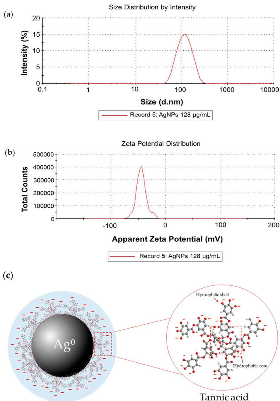
**Figure 2.** Dynamic Light Scattering (DLS) measurement of silver nanoparticles (AgNPs): (a) size distribution graph of AgNPs at  $101.13 \pm 0.85$  nm; (b) and zeta potential of AgNPs at  $-47.63 \pm 5.79$  mV; (c) the simple structural model of tannic acid stabilized AgNPs molecules (pH = 5.94).
