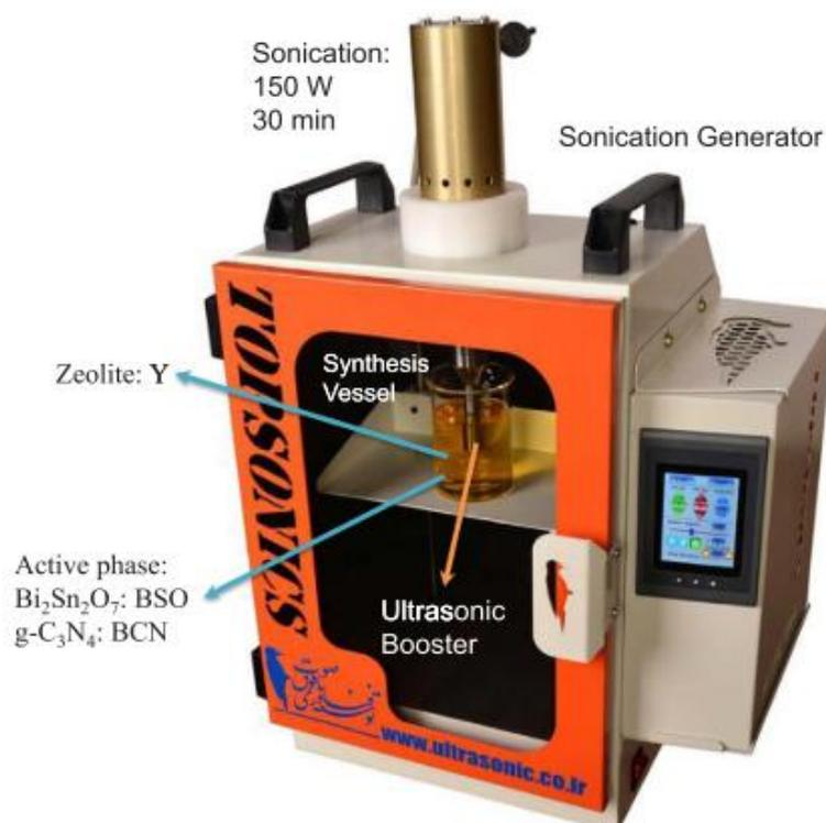
**Figure 16.** Experimental setup for the sono-dispersion of bulk  $Bi_2Sn_2O_7$  and  $g-C_3N_4$  over zeolite Y. Reprinted with permission from [50].
