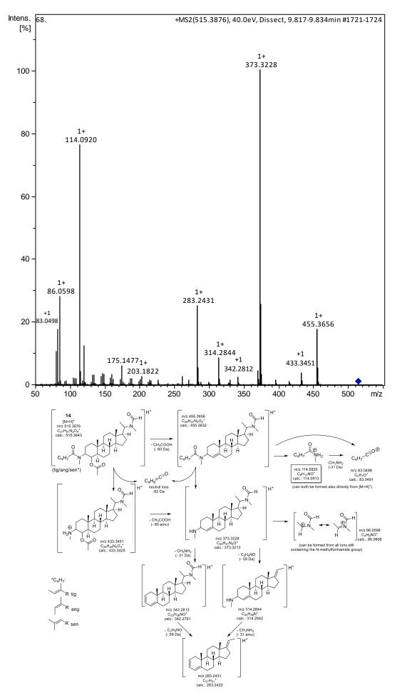
**Figure S14.** (+)ESI MS<sup>2</sup> spectrum and fragmentation pathway for the  $[M+H]^+$  ion of compound 14 at m/z 515.3876.Note that the acetoxy group could also be at C-2. (Spectrum taken from fraction A5G).
