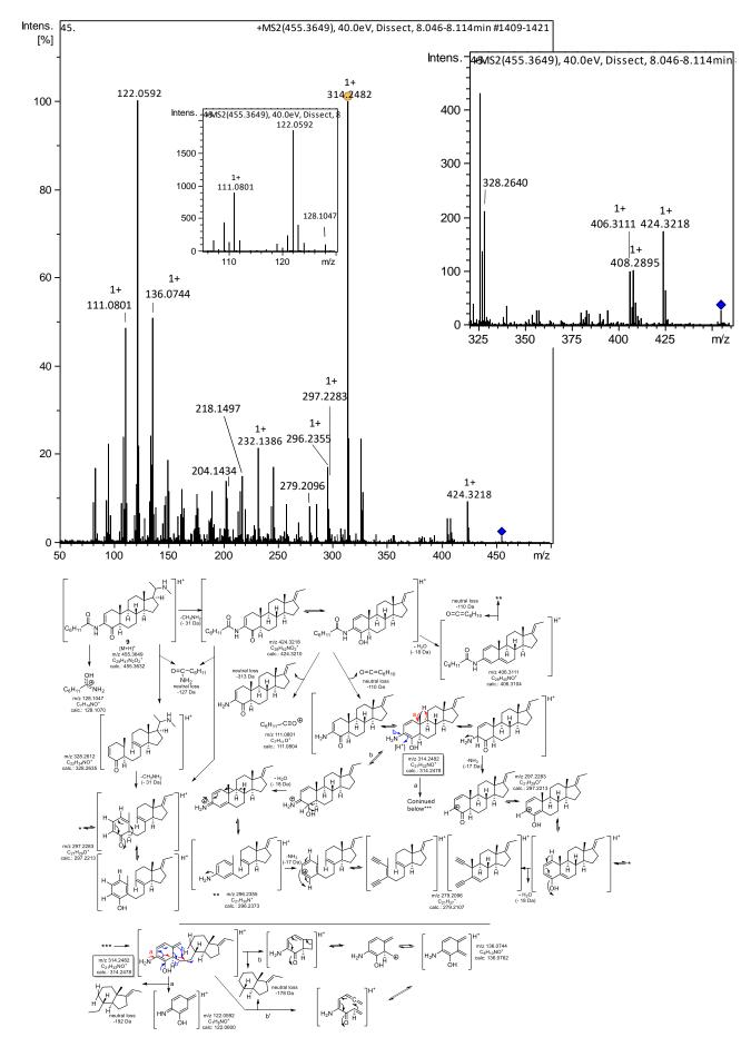
**Figure S9.** (+)ESI MS<sup>2</sup> spectrum and fragmentation pathway for the  $[M+H]^+$  ion of compound **9** at m/z 455.3649. (Spectrum taken from fraction A5D).
