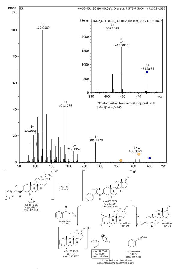
**Figure S8.** (+)ESI MS<sup>2</sup> spectrum and fragmentation pathway for the  $[M+H]^+$  ion of compound **8** (Epipachysamine D [9, 10] at m/z 451.3689. (Spectrum taken from fraction A5).
