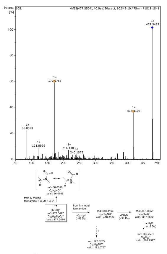
**Figure S17.** (+)ESI MS<sup>2</sup> spectrum and fragmentation pathway for the  $[M+H]^+$  ion of compound **17** at *m/z* 477.3504. (Spectrum taken from fraction A5P).
