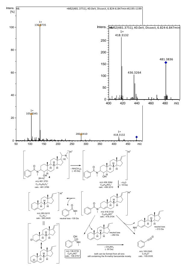
**Figure S4.** (+)ESI MS<sup>2</sup> spectrum (top: full mass range, bottom: magnified high m/z region) and fragmentation pathway for the [M+H]<sup>+</sup> ion of compound **4** at m/z 481.3751 (note that the OH group was postulated at C-4 in analogy to the known acetate **6**, compare with Figure S5). (Spectrum taken from fraction 3C).
