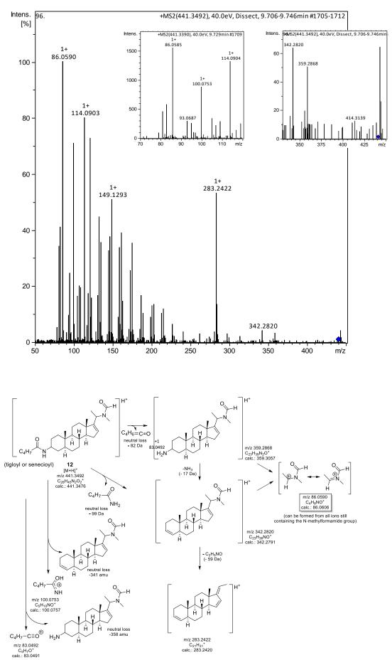
**Figure S12.** (+)ESI MS<sup>2</sup> spectrum and fragmentation pathway for the  $[M+H]^+$  ion of compound **12** at m/z 441.3492. (Spectrum taken from fraction A5P).
