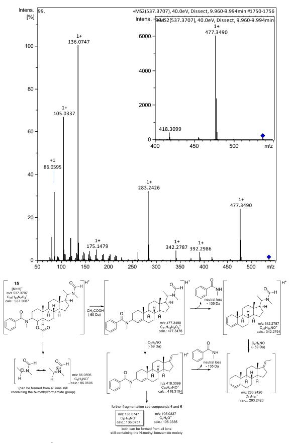
**Figure S15.** (+)ESI MS<sup>2</sup> spectrum and fragmentation pathway for the  $[M+H]^+$  ion of compound **15** at m/z 537.3707 (note that the acetate moiety could also be at C-2).(Spectrum taken from fraction A5P).
