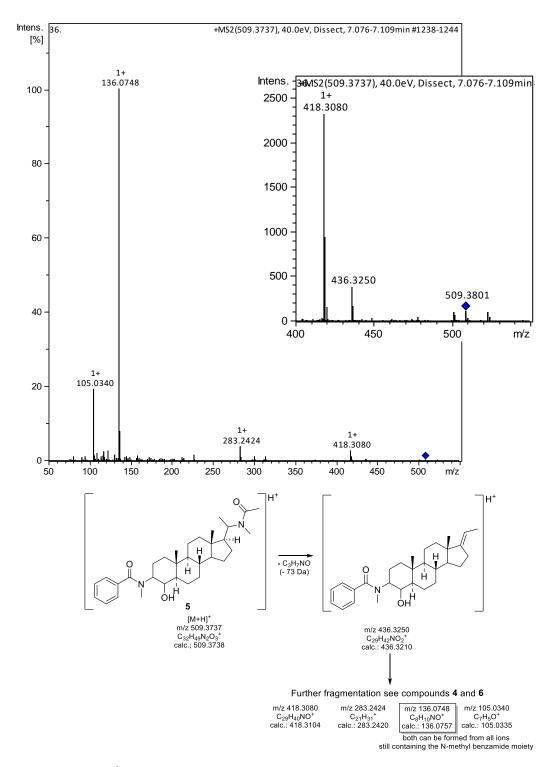
**Figure S5.** (+)ESI MS<sup>2</sup> spectrum and fragmentation pathway for the  $[M+H]^+$  ion of compound **5** at *m/z* 509.3737. (Spectrum taken from fraction A5H).
