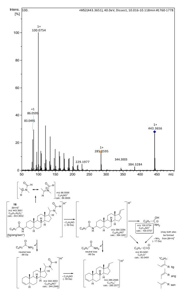
**Figure S16.** (+)ESI MS<sup>2</sup> spectrum and fragmentation pathway for the  $[M+H]^+$  ion of compound **16** at m/z 443.3651. (Spectrum taken from fraction A5P).
