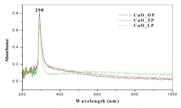
Figure 1. UV-Vis spectra of CuONPs from citrus peels extracted with distilled water solvent.
