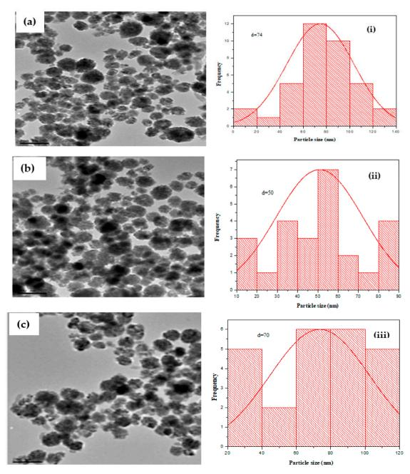
**Figure 8.** TEM images for (**a**) CuO-NPs-ODI, (**b**) CuO-NPs-LDI and (**c**) CuO-NPs-TDI from orange, lemon and tangerine extracts, respectively, using distilled water as solvent and their size distribution histogram. (**i**) CuO-NPs-ODI, (**ii**) CuO-NPs-LDI and (**iii**) CuO-NPs-TDI.
