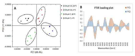
**Figure 1.** Principal components score plot (**A**) and loading plot (**B**) of β-casein of the FTIR spectra in region 1700–1600 cm<sup>-1</sup> where β-casein at pH 5.9 and temperature of 20 °C (black), β-casein at pH 5.9 and temperature of 4 °C (red), β-casein at pH 7.0 and temperature of 20 °C (green) and β-casein at pH 7.0 and temperature of 4 °C (blue) are in (**A**) and PC1 (orange) and PC2 (blue) are in (**B**).
