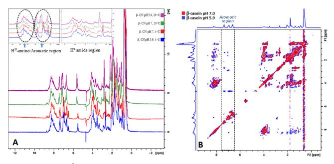
Figure 2. (A) Overlayed  $^1H$  NMR spectra of β-casein at pH 5.9 and temperature of 20  $^{\circ}$ C (purple), β-casein at pH 5.9 and temperature of 4  $^{\circ}$ C (blue), β-casein at pH 7.0 and temperature of 20  $^{\circ}$ C (green) and β-casein at pH 7.0 and temperature of 4  $^{\circ}$ C (red). (B) Overlayed TOCSY NMR spectra of β-casein at pH 7.0 (red) and β-casein at pH 5.9 (blue).
