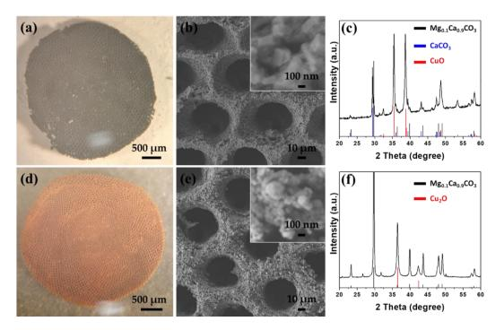
**Figure 4.** Structural characterization of the 3D structure after converting the hydroxide shell to an oxide. (**a**,**d**) The optical images, (**b**,**e**) SEM images, and (**c**,**f**) XRD patterns of *Sorites*@CuO and *Sorites*@Cu<sub>2</sub>O, respectively. The black, blue, and red stick patterns in the XRD panels correspond to the rhombohedral  $Mg_{0.1}Ca_{0.9}CO_3$ , rhombohedral  $CaCO_3$ , and the coated materials, respectively.
