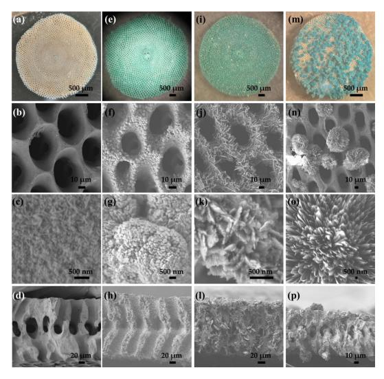
**Figure 2.** Optical and scanning electron microscopy (SEM) images of the *Sorites* 3D structure before (left column, **a**–**d**) and after reacting with three different copper salts (the subsequent columns from left to right): CuCl<sub>2</sub> (**e**–**h**), Cu(NO<sub>3</sub>)<sub>2</sub> (**i**–**l**), and Cu(ac)<sub>2</sub> (**m**–**p**). (**a**,**e**,**i**,**m**) optical images, SEM top-view images, and SEM cross-section images (**d**,**h**,**l**,**p**).
