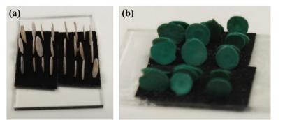
**Figure 1.** Optical images of the *Sorites* before (**a**) and after (**b**) reacting with  $CuCl_2$  to form a 3D structure of copper-based hydroxide.
