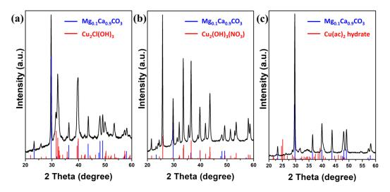
**Figure 3.** X-ray diffraction patterns of the 3D structures after reacting *Sorites* with different copper salts. (a) *Sorites*@Cu<sub>2</sub>Cl(OH)<sub>3</sub>, (b) *Sorites*@Cu<sub>2</sub>(OH)<sub>3</sub>(NO<sub>3</sub>), and (c) *Sorites* decorated with Cu(ac)<sub>2</sub> hydrate. The blue and red bars in the XRD panels correspond to the rhombohedral Mg<sub>0.1</sub>Ca<sub>0.9</sub>CO<sub>3</sub> and the coated material, respectively.
