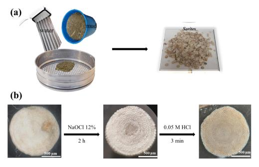
**Figure 6.** Purification and pretreatment processes of *Sorites*: (**a**) sifting and washing, (**b**) chemical pretreatment.
