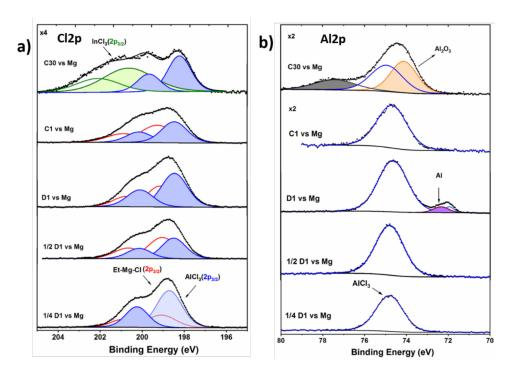
Figure 5. (a) Cl2p and (b) Al2p core peaks spectra of the InSb electrodes cycled in EtMgCl-Et<sub>2</sub>AlCl/THF electrolyte vs. Mg.
