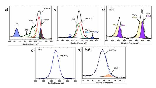
**Figure 6.** (a) C1s, (b) O1s/Sb3d, (c) In3d, (d) F1s, and (e) Mg2p core peaks spectra of slightly demagnesiated InSb in 0.5 M Mg(TFSI)<sub>2</sub>/DME electrolyte.
