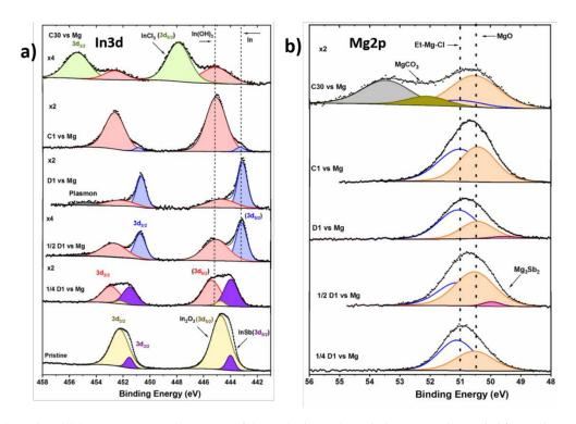
**Figure 4.** (a) In3d and (b) Mg 2p core peaks spectra of the InSb electrode cycled in EtMgCl–Et2AlCl/THF electrolyte vs. Mg. All spectra were calibrated by considering the adventitious carbon peak (C-C/C-H) at 284.8 eV.
