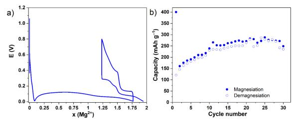
**Figure 1.** (a) Galvanostatic profiles and (b) capacities upon cycling for InSb/Mg cells cycled at C/50 rate between 0.8 and 0.005 V in 0.35 M EtMgCl–Et<sub>2</sub>AlCl/THF.
