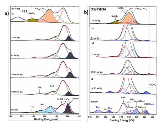
**Figure 3.** (a) C1s and (b) O1s/Sb3d core peaks spectra of the InSb electrode cycled in EtMgCl–Et2AlCl/THF electrolyte vs. Mg.  $\frac{1}{4}$ D1,  $\frac{1}{2}$ D1, D1, C1, and C30 denote the first one-quarter discharge, first half discharge, first discharge, first charge, and 30th charge, respectively. All spectra were calibrated by considering the adventitious carbon peak (C-C/C-H) at 284.8 eV.
