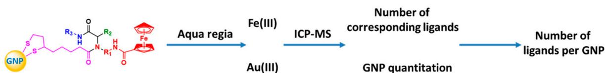
**Scheme 2.** One step determination of the number of ligands per GNP. The concentrations of Au(III) and Fe(III) were quantitatively determined by ICP-MS. The concentration of total GNPs was determined according to the Au content, and the total number of ligands was determined according to the Fe content. The loaded ligands per nanoparticle could then be obtained.
