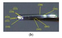
Figure 4. Face indexation data of (a) ST-A and (b) ST-B.
