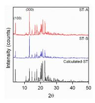
**Figure 3.** Overlay of PXRD patterns of ST-A, ST-B, and calculated ST.
