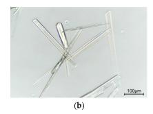
**Figure 2.** Compound micrographs of the crystal habit of Sor-Tos crystals grown from (**a**) acetone and (**b**) n-butanol.
