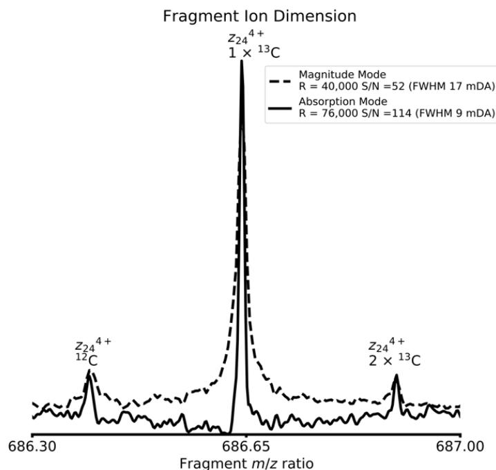
**Figure 2.** Extracted fragment ion scan from the 2D mass spectrum for the  $1 \times {}^{13}\text{C}$  isotope of  $[\text{M} + 6\text{H}]^{6+}$  ions of the monomethylated histone peptide (K7 1m) at  $m/z$  489.453, zoom-in on fragment ion  $z_{24}^{4+}$ , comparison between absorption mode and magnitude mode.
