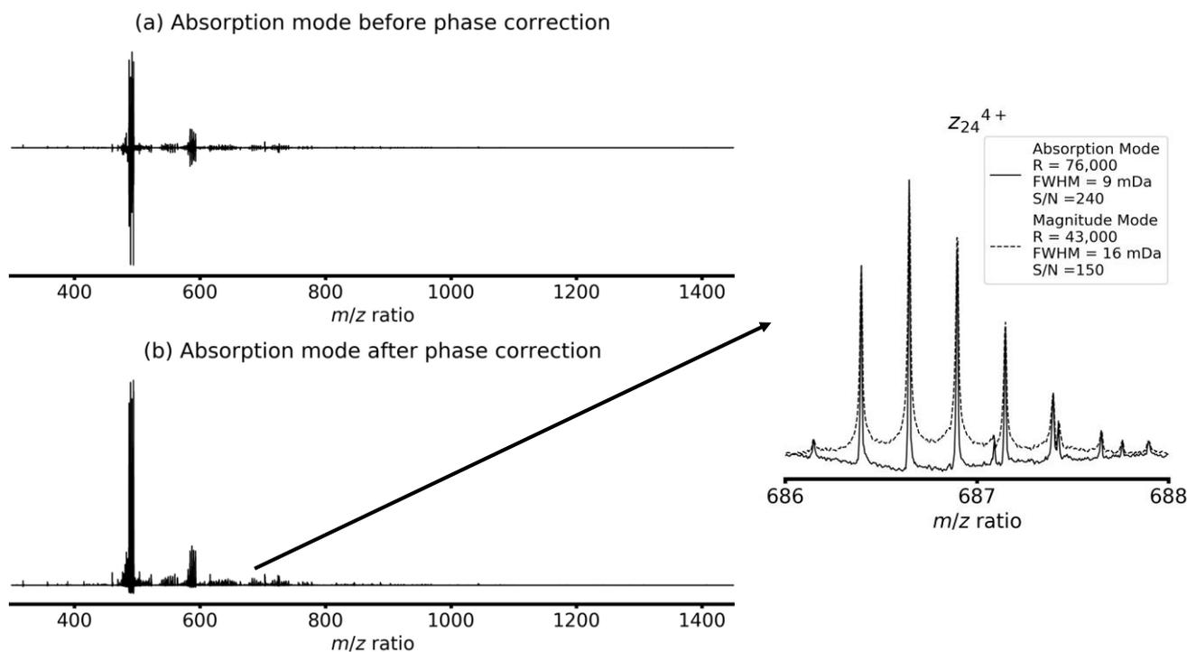
**Figure 1.** Tandem mass spectrum of the  $[M + 6H]^{6+}$  histone peptides with ECD fragmentation in absorption mode (a) before phase correction and (b) after phase correction. Insert: zoom-in on the  $z_{24}^{4+}$  fragment ion isotopic distribution of the monomethylated histone peptide (K7 1m), comparison between magnitude mode and phase-corrected absorption mode (FWHM: full-width at half-maximum).
