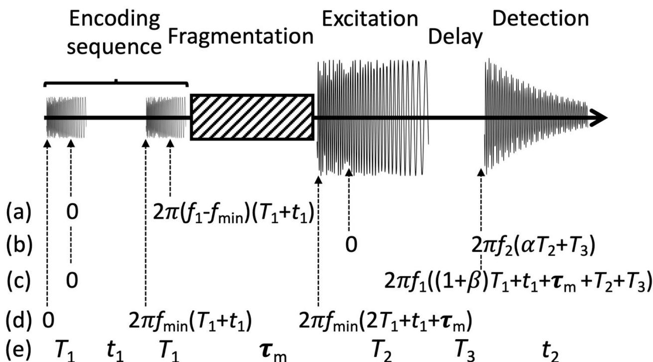
**Scheme 1.** Pulse sequence for two-dimensional mass spectrometry and evolution of phases for (a) precursor ion radii, (b) fragment ion motion, (c) unfragmented precursor ion motion, (d) excitation pulses. (e) Duration of each segment of the pulse sequence. The factor  $\alpha$  (resp.  $\beta$ ) is related to the moment that the swept frequency of the chirp reaches the cyclotron frequency of the fragment (resp. unfragmented precursor).
