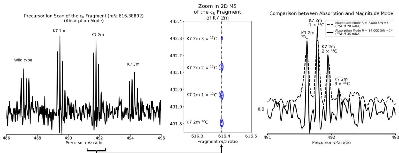
**Figure 3.** Precursor ion scan extracted from the absorption mode 2D mass spectrum for the  $^{12}\text{C}$  isotope of the  $c_6$  fragment of the histone peptides ( $m/z$  616.38892), zoom-in on the  $c_6$  fragment ion isotopic distribution in the 2D mass spectrum for the dimethylated histone peptide (K7 2m), comparison between the absorption mode and magnitude mode of the precursor ion scan of the  $c_6$  fragment.
