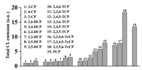
**Figure 3.** Intrinsic •OH-dependent CL were also generated from all 19 chlorophenols in AOPs mediated by Fe(II)-Fenton system [48]. The CL emission was measured by an ultraweak CL analyzer, and the intensity of total CL emission was recorded. CPs, 10 µM; Fe(II)–EDTA, 1 mM; H<sub>2</sub>O<sub>2</sub>, 100 mM. Copyright © 2015, American Chemical Society.
