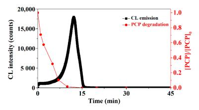
**Figure 2.** The CL emission from PCP/Fenton system correlated well with PCP degradation [48]. The CL emission was measured by an ultraweak CL analyzer, with the CL signal recorded at a time interval of 0.1s. The kinetics of PCP degradation was monitored by HPLC analysis. For detailed experimental procedure, please refer to our previous study [48]. PCP, 1 mM; Fe(II)–EDTA, 3 mM; H<sub>2</sub>O<sub>2</sub>, 300 mM. Copyright © 2015, American Chemical Society.
