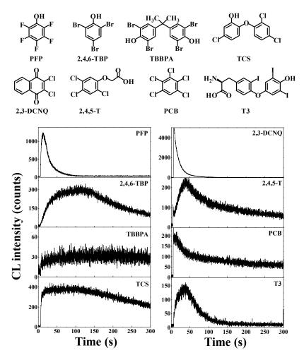
**Figure 5.** Similar •OH-dependent intrinsic CL were also produced from the degradation of several typical XAr in classic Fe(II)-Fenton system [48]. The CL emission was measured by an ultraweak CL analyzer, with the CL signal recorded at a time interval of 0.1 s. PFP, 2,4,6-TBP, TBBPA, TCS, 2,4,5-T and PCB, 30  $\mu$ M; 2,3-DCNQ, 30  $\mu$ M; T3, 3  $\mu$ M; Fe(II)–EDTA, 1 mM; H<sub>2</sub>O<sub>2</sub>, 100 mM. Copyright © 2015, American Chemical Society.
