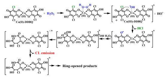
**Scheme 2.** The potential molecular mechanism for the unexpectedly strong CL emission from DDBQ/Co(II)-Fenton-like system mainly depends on site specifically produced •OH [51]. Copyright 2020, with permission from Elsevier.
