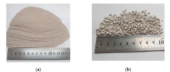
**Figure 7.** Photograph of the: (**a**) zeolitic by-product; (**b**) coarser fraction of sorption material based on straetlingite.
