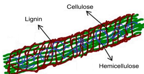
**Figure 6.** Hierarchical structure of lignocellulosic biomass.
