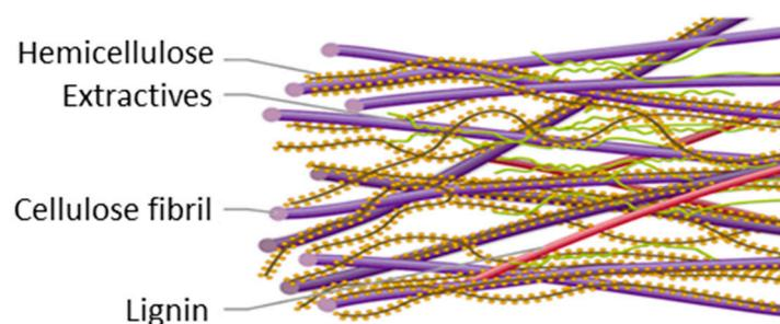
**Figure 2.** Illustration of the distribution of the lignin and carbohydrates in the fiber surface.
