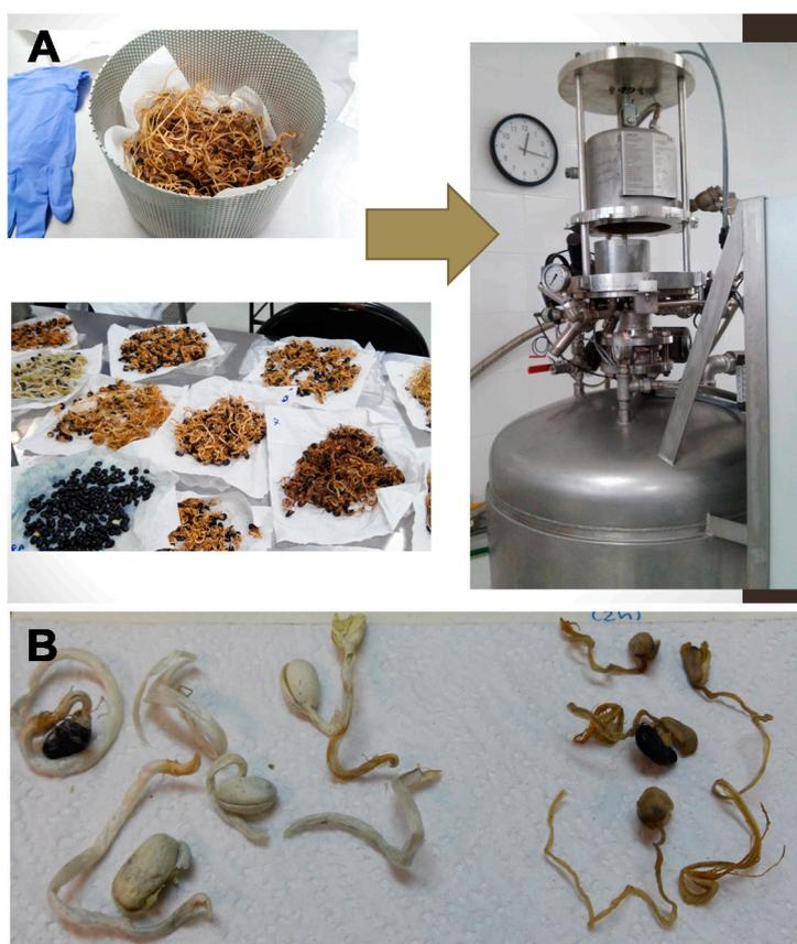
**Figure 10.** (A) Instant controlled pressure drop treatment. (B) DIC5, germinated beans treated under 0.27 MPa during 70 s.
