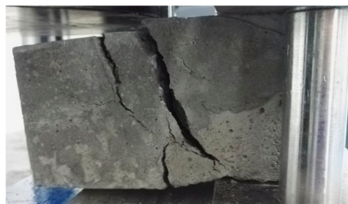
Figure 3. The failure mode of interface with the steel bar.
