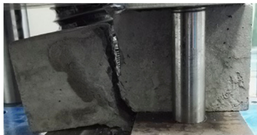
Figure 4. The failure mode of interface without the steel bar.
