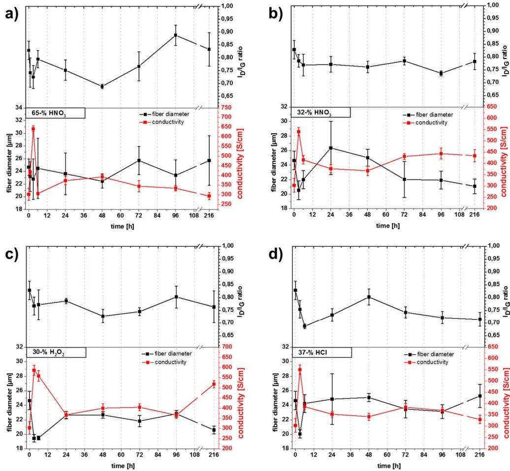
**Figure 9.** Conductivity,  $I_D/I_C$  ratio and fiber diameter of CNY after different acidification times: (a) concentrated nitric acid, (b) half concentrated nitric acid, (c) concentrated hydrogen peroxide and (d) concentrated hydrochloric acid.
