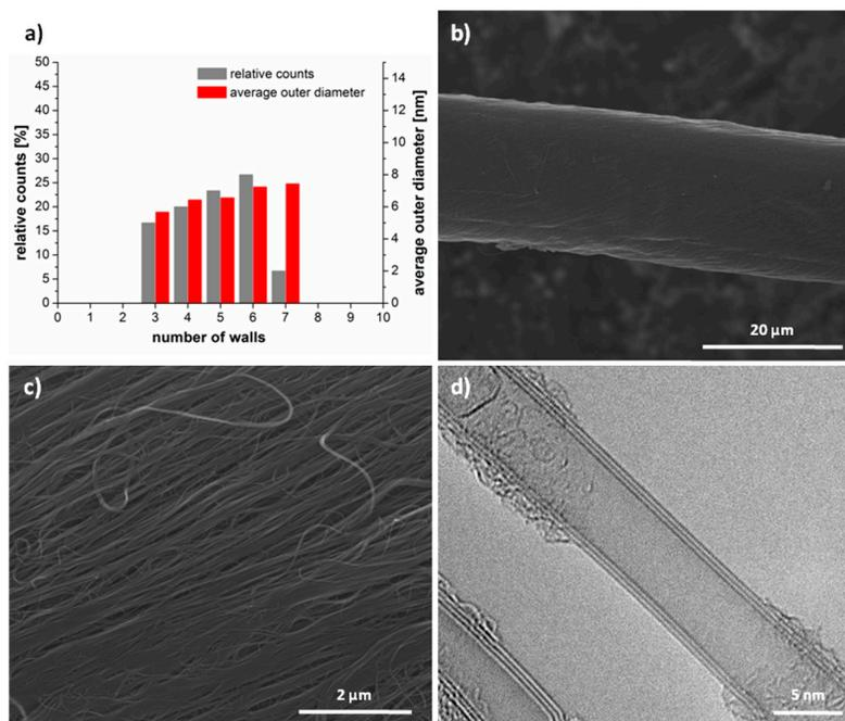
**Figure 2.** Investigation of CNY annealed for 2 h at 2500 °C. (a) Statistical analysis of the annealed CNT, (b) and (c) SEM images of annealed CNY and (d) TEM image of annealed CNT.
