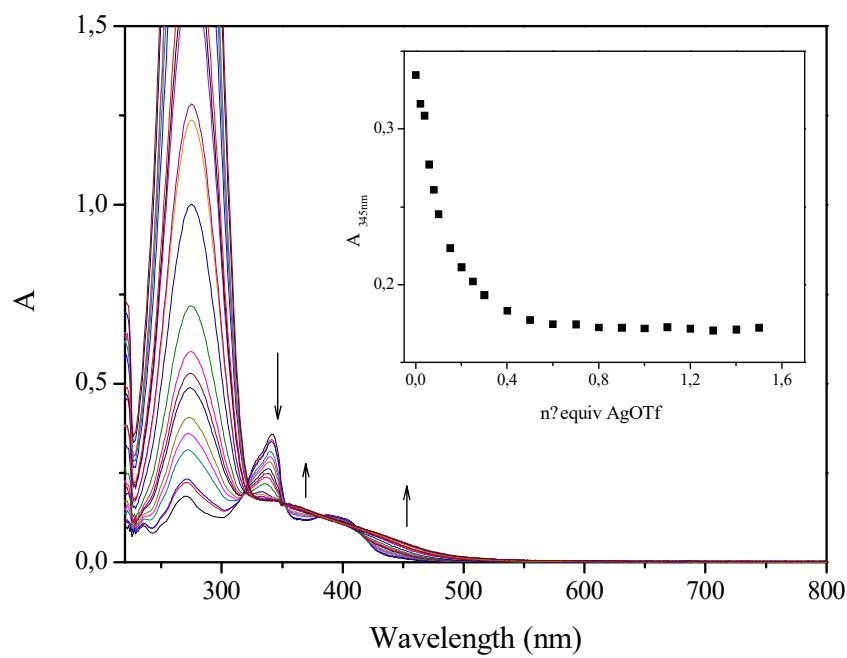
**Figure S11.** Absorption spectra of  $1 \cdot 10^{-5}$ M dichloromethane solution of **4** upon addition of increasing amounts of AgOTf. Inset: variation of absorption maxima at 345 nm each titration point.
