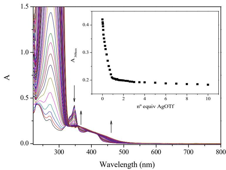
**Figure S9.** Absorption spectra of  $1 \cdot 10^{-5}$ M dichloromethane solution of **3** upon addition of increasing amounts of AgOTf. Inset: variation of absorption maxima at 348 nm each titration point.
