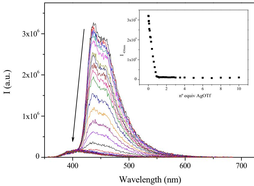
**Figure S10.** Emission spectra of  $1 \cdot 10^{-5}$ M dichloromethane solution of **3** upon addition of increasing amounts of AgOTf. Inset: variation of emission maxima at 436 nm at each titration point.
