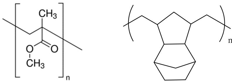
**Figure S12.** Chemical structure of PMMA, with MW = 996.00 kDa (left) and Zeonex 480R, with MW = 480 kDa (right).
