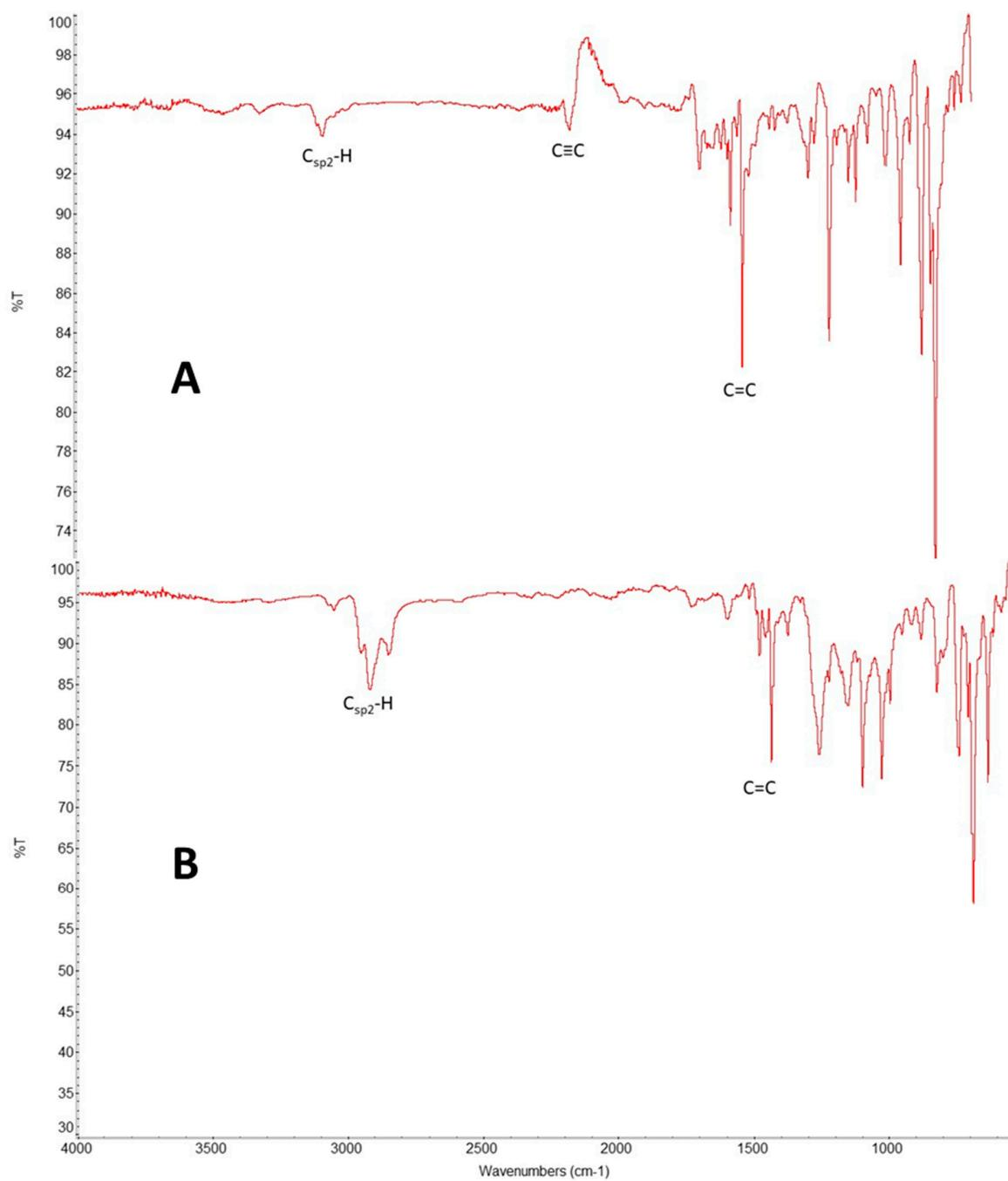
**Figure S18.** IR spectra of **3** (A) and **3·Ag** (B).
