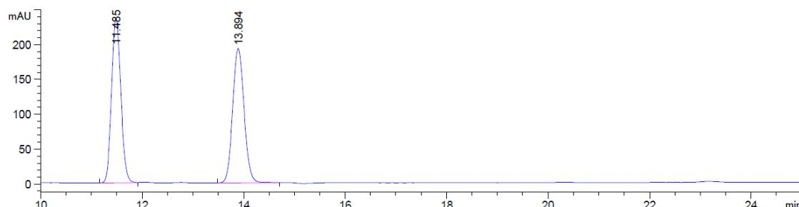
**Bioreduction using KRED-P2-D11 for the production of (*R*)-alcohol **3b** in 99% ee**
