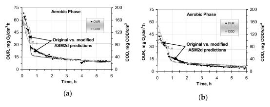
**Figure 2.** Measured data vs. the original (solid lines) and the modified (shaded lines) ASM2d after optimization step for OUR batch tests in two parallel reactors with mixed liquor from Wschod WWTP: (a) the SWW without pretreatment and (b) the SWW after C–F.
