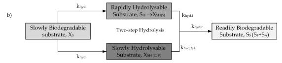
**Figure 4.** The concept of one/two-steps hydrolysis model based on the original (**a**) vs. the modified (Activated Sludge Model No 2d) ASM2d that was proposed by Drewnowski and Makinia [26] (**b**) and verified by Makinia and Czerwionka [39], as well as by Maruéjouls et al. [47], depending on chemical oxygen demand (COD) forms/molecule size. Note: More details regarding the two-step hydrolysis might be found in Table S1 in Supplementary Materials.
