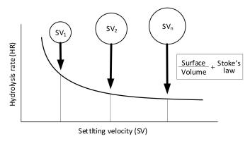
**Figure 5.** The hydrolysis rate constants in regard to the particle settling velocity (SV) according to the model that was proposed by Maruéjouls et al. [52].
